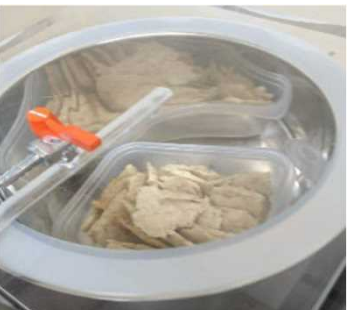
Freeze minced sample into thin plates
