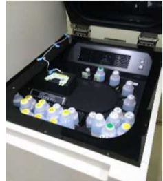
Measure the radiation with Liquid scintillation counter
