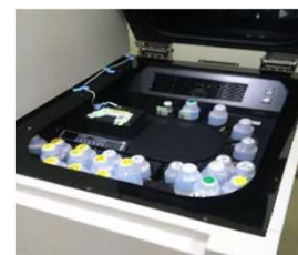
Measure the radiation with Liquid scintillation counter
