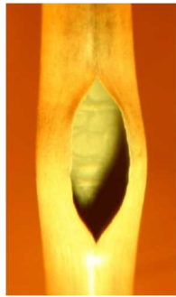
(a) LOCA 模擬試験後の被覆管 36 (a) Cladding tube after LOCA test
