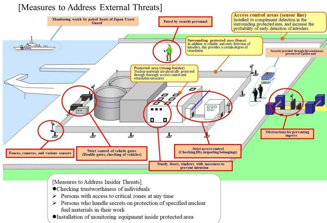
Figure 3-1: Overview of Protection Measures for Nuclear Facilities
