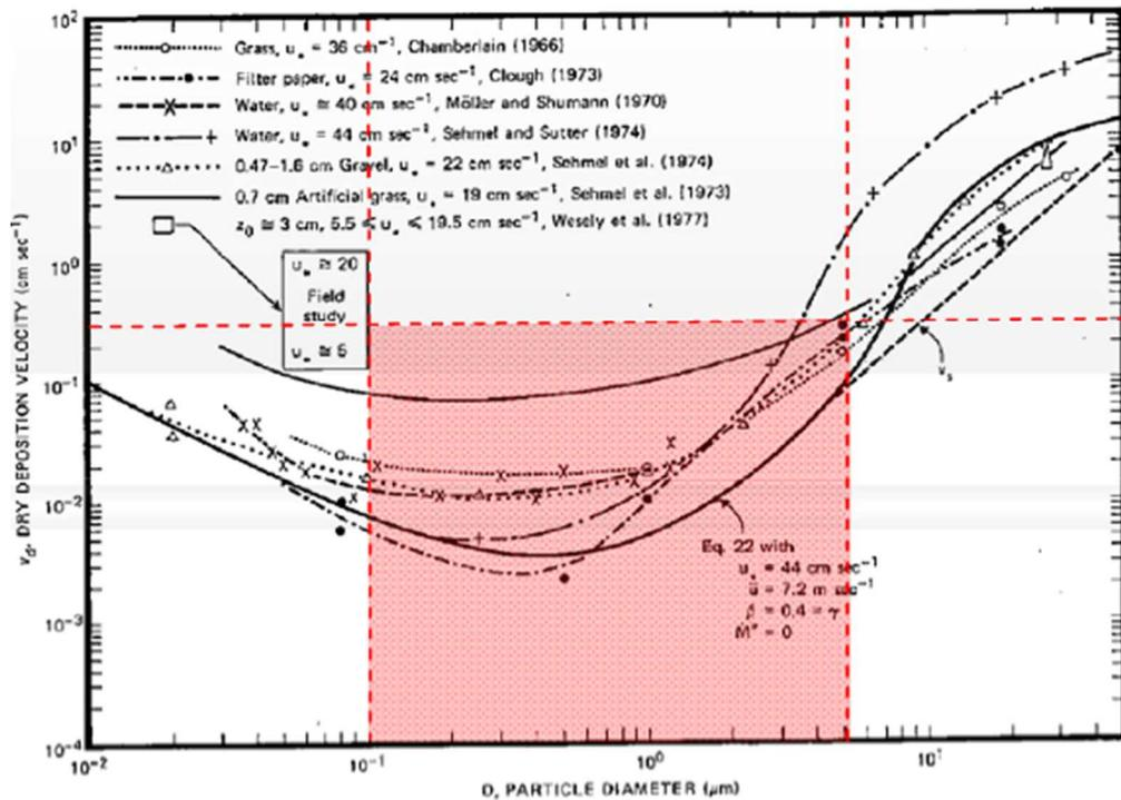
Fig. 4 Dry deposition velocity as a function of particle size. Data were obtained from a number of publications.<sup>19-24</sup> The theoretical curve appropriate for a smooth surface is shown for comparison. Note that the theoretical curve is strongly dependent on the value for  $u_*$  and that Eq. 22 does not contain a parameterization for surface roughness. For a preliminary study of the effect of surface roughness and other factors, see Ref. 5.
