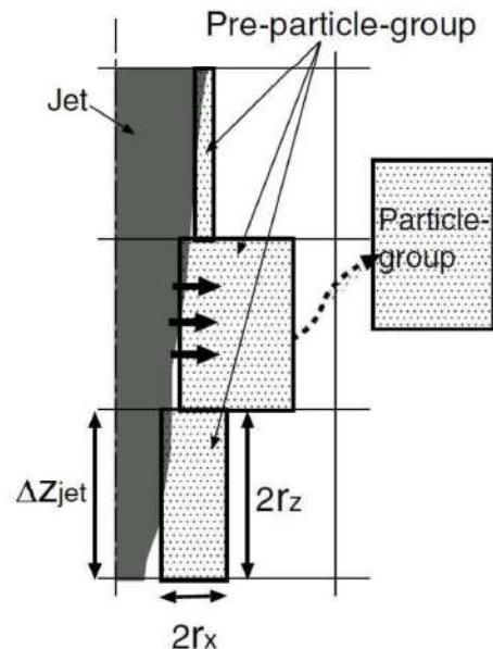
図2-6 融体粒子モデル概要図<sup>(1)</sup>
