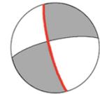
走向 = $165^\circ$<br>すべり角 = $-15^\circ$<br>傾斜角 = $80^\circ$   |
