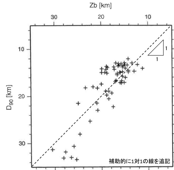
Fig. 8. Plot of the depth to the basal depth of magnetic sources ( $Z_b$ ) against the seismicogenic layer thickness ( $D_{90}$ ) beneath the Japanese islands.磁化層下限値( $Z_b$ )とD90%の関係
