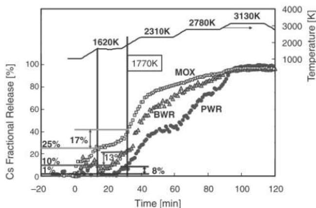
**Fig. 3** Fuel temperature and fractional releases of Cs
