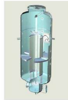
Fig. 5-4: THAI test vessel
