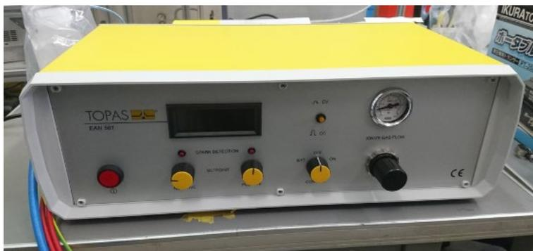
(a) Electrostatic aerosol neutralizer
