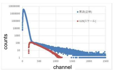
β-ray spectrometry of the water at Expand ALPS outlet β-ray spectrometry of H4N-A6 tank water
