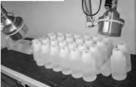
Figure 5.3: Bottle phantom (70-kg-configuration) in the WBC.
