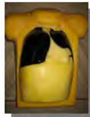
LLNL phantoms ^{241}\text{Am}+^{152}\text{Eu} , ^{238}\text{Pu}+^{239}\text{Pu}+^{241}\text{Am} each
