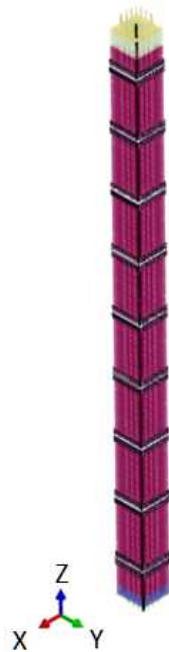
図2.11 燃料集合体有限要素法モデルの概観 Fig. 2.11 Appearance of the FEM model of a fuel assembly
