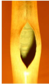
(a) LOCA 模擬試験後の被覆管 23 (a) Cladding tube after LOCA test
