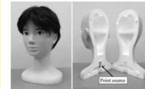
Figure 2. A manikin head used for the exercise in which point source was installed to imitate 131 I thyroid content.
