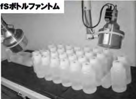
Figure 5.3: Bottle phantom (70-kg-configuration) in the WBC.
