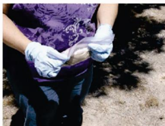
Roll the bag around the soil. Keep the opening away from breathing area
