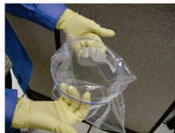
Clean Person: Roll the bag until a lip has been created. Hold bag under lip ensuring that the bag remains open for the (dirty person) to place the sample into the bag, without touching the outside of the bag.
