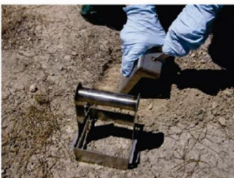
Dig trench with trowel, use claw hammer if needed to loosen soil.
