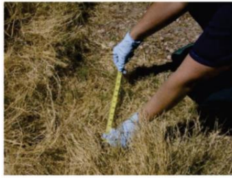
Measure the Length, Width and Depth of the sample collected
