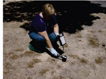
Survey Area Exposure Rate (waist high) & Contamination (ground). Record as a measurement.
