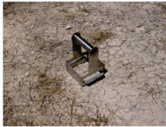
Place jig at sample location, with as little vegetation as possible. If vegetation is present, remove as much vegetation as possible.
