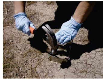
Push Jig to 2 cm depth. Tap with Hammer if needed.
