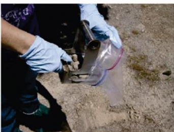
Pick up Jig and Trowel with the sample. Pour content into 1 gallon Sealable Bag
