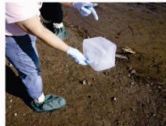
Collect a small amount of sample water and rinse out the sample container.
