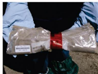
Place a SCF barcode & Security Seal on the bag. Complete the Sample Control & Chain of Custody Form and input into the Tablet If Background permits survey the Sample and record on SCF.
