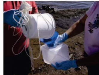
Using the funnel fill the 1 liter container. Stop 1 inch from the top
