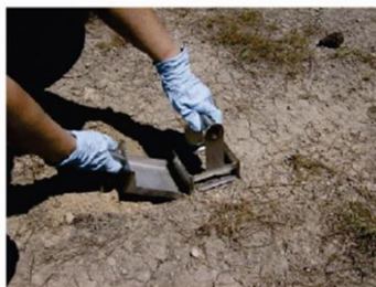
Slide Trowel under jig, use hammer if necessary to push trowel under the jig.
