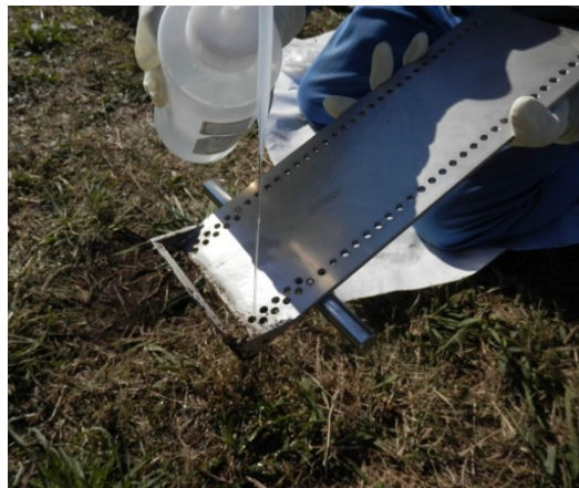
Figure E.9 Cleaning sampling tools
