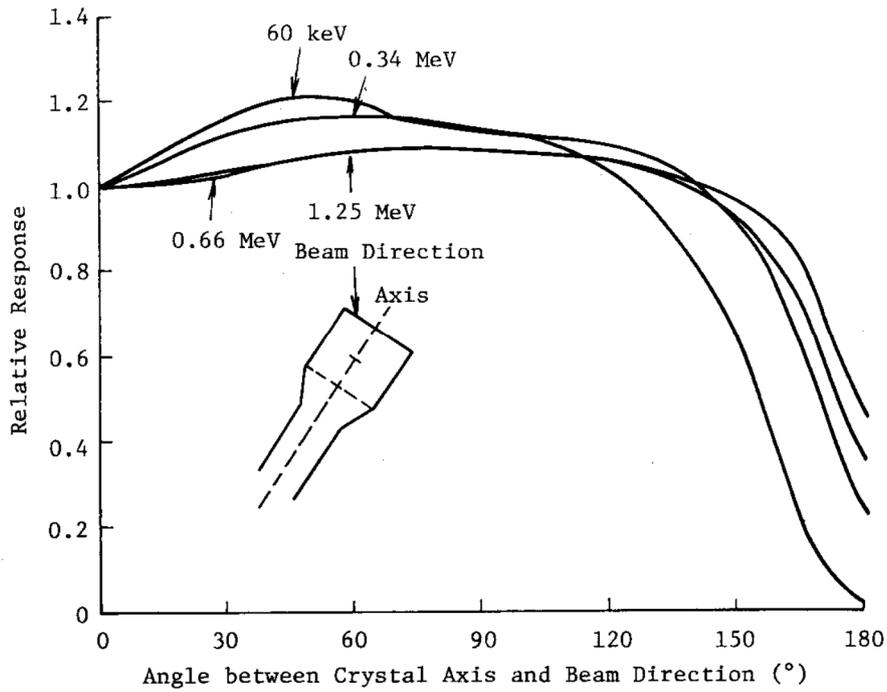
Figure B.6 Example of directional characteristics of NaI (Tl) scintillator (3 in.  $\phi$   $\times$  3 in. cylindrical)
