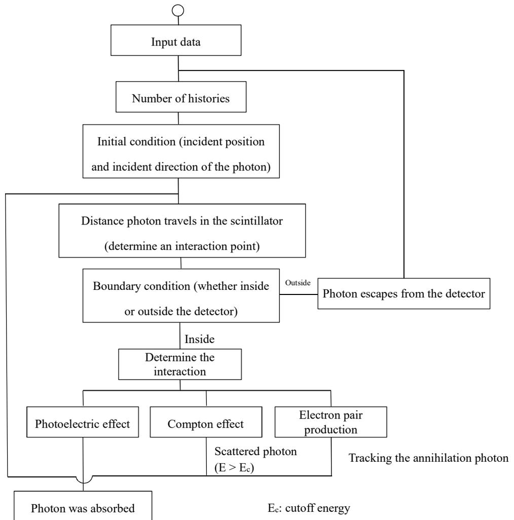
Figure J.3 Flowchart of creating a response function by the Monte Carlo simulation method (simplified)
