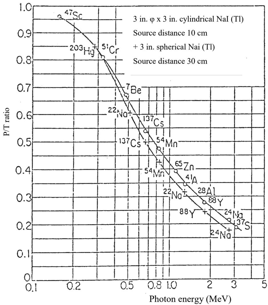
Figure 2.1 P/T ratio of NaI (Tl) scintillator
