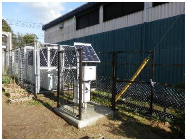
Figure 5.5 Example of the installation status of a simplified electronic dosimeter
