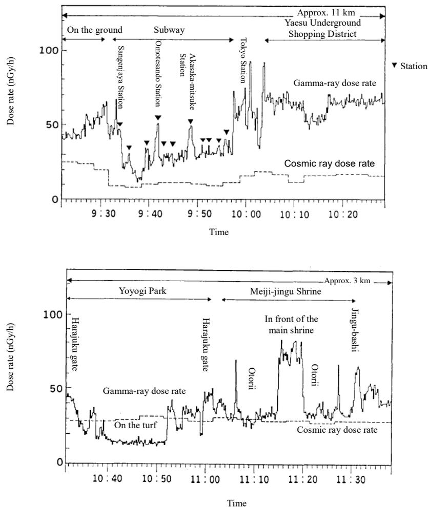
Figure G.4 Examples of variations in dose rate due to changes in the surroundings (Reference 18)
