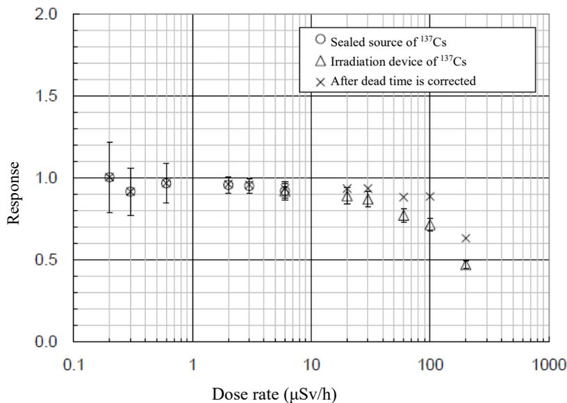
Figure B.14 Dose rate linearity in a CsI (Tl) scintillation detector
