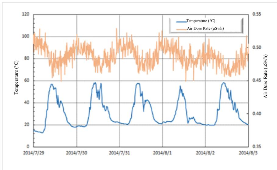
Figure E.4 Effect of temperature changes during continuous measurement by a transportable monitoring post (silicon semiconductor)
