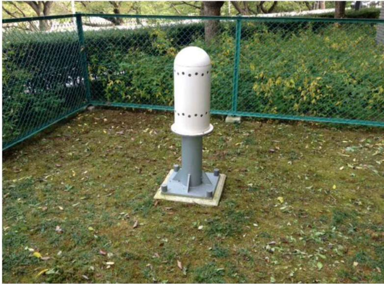
Figure 5.1 Example of installation on an alley, at a height of 1 m above the ground (Aichi Prefecture)
