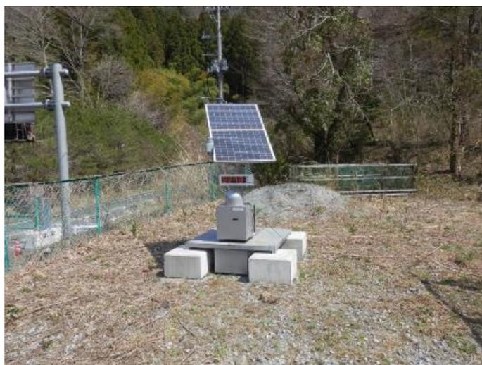
Figure 5.6 Example of the installation status of a transportable monitoring post (the positioning of the detector: 1 m above the ground, with solar power generation and external battery facilities)
