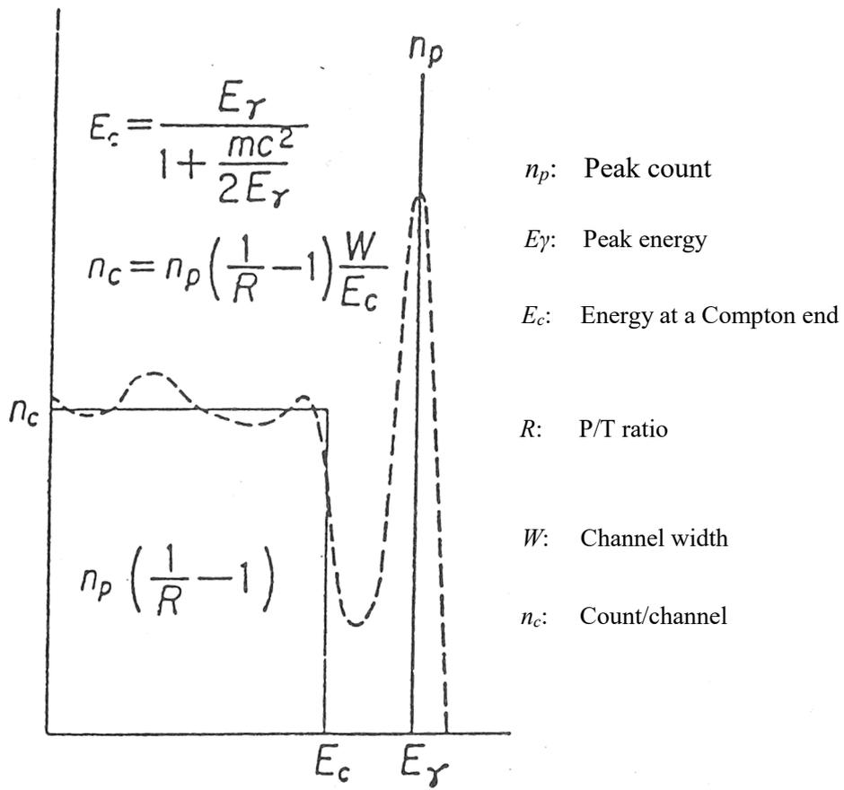
Figure 2.2 Subtraction method for a Compton continuum
