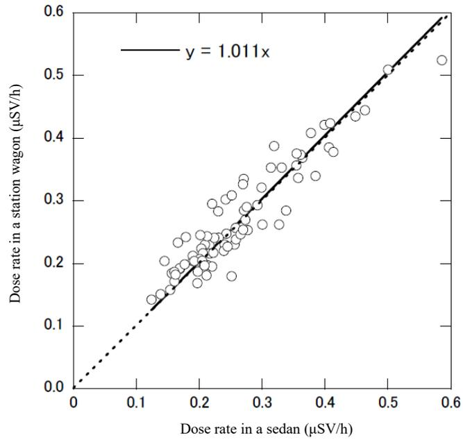
Figure F.4 Comparison of dose rates between vehicle types (a station wagon and a sedan)
