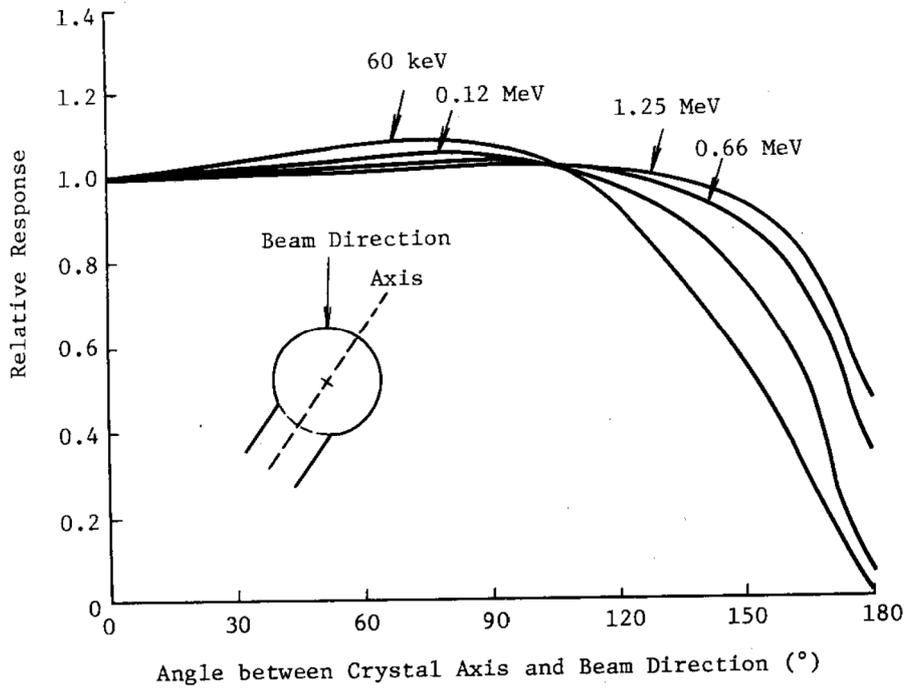
Figure B.7 An example of directional characteristics of NaI (Tl) scintillator (3 in.  $\phi$  spherical)
