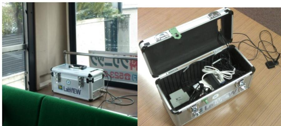
Figure 5.8 Example of a portable type (left: when installed; right: inside of the storage case)
