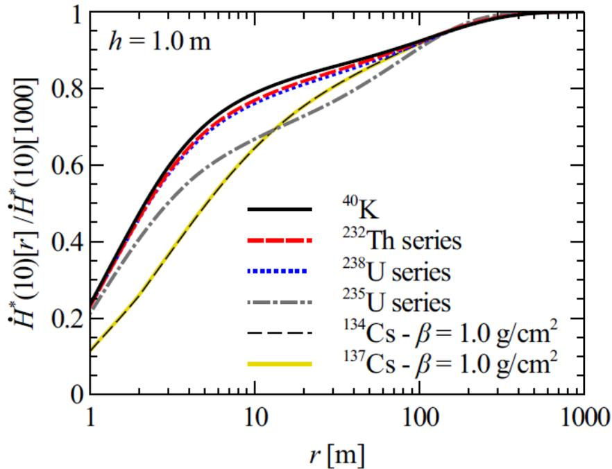
Figure F.1 Contribution ratio from the surroundings with regard to the ambient dose equivalent at 1 m above ground when natural radionuclides are uniformly distributed in the ground and  $^{134}\text{Cs}$  and  $^{137}\text{Cs}$  are exponentially distributed ( $\beta: 1.0 \text{ g/cm}^2$ ) (Reference 17)
