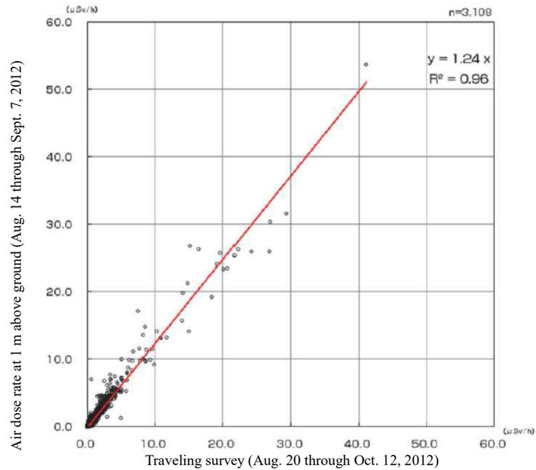
Figure F.2 Relationship between the measurement results by a traveling survey system (mean values in a 100-m square mesh) and the dose rate around the travel route (Reference 15)
