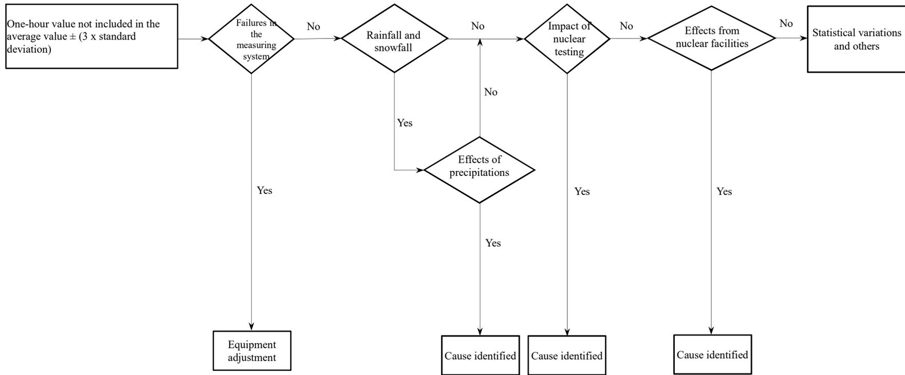
Figure 7.1 Example of a flowchart for outlier analysis
