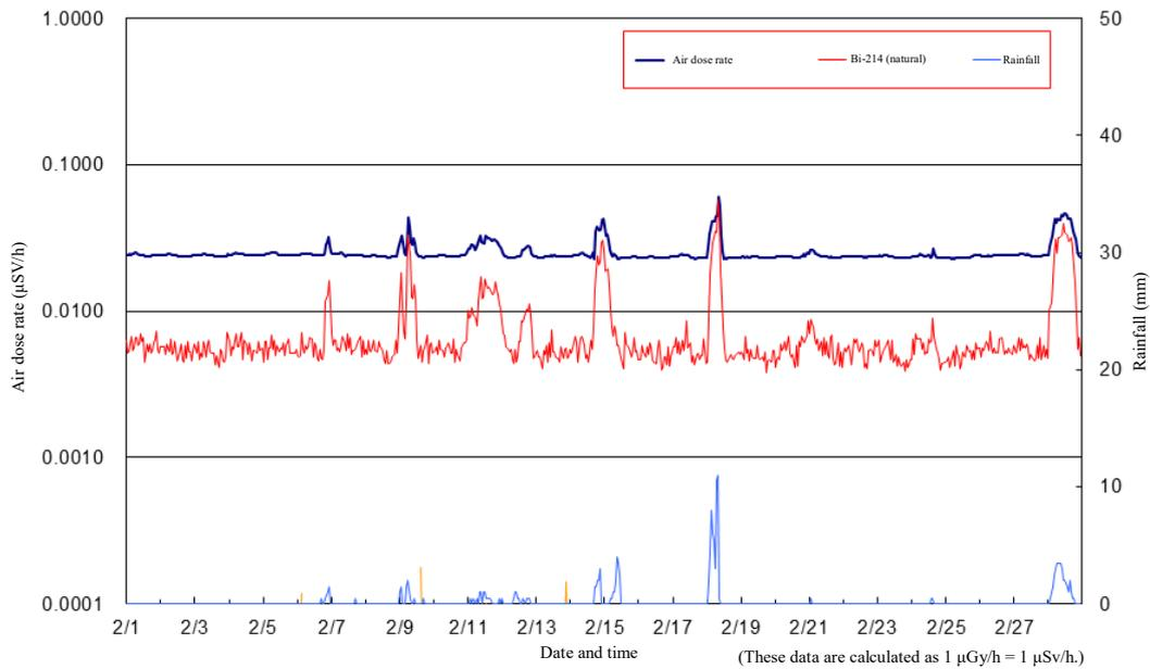
Figure G.2 Example of an increase in the air dose rate due to rainfall
