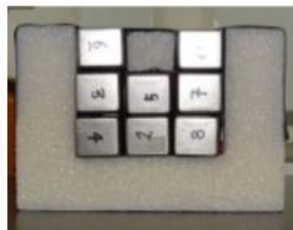
GAGG monitor (assembled 8 GAGG modules)
