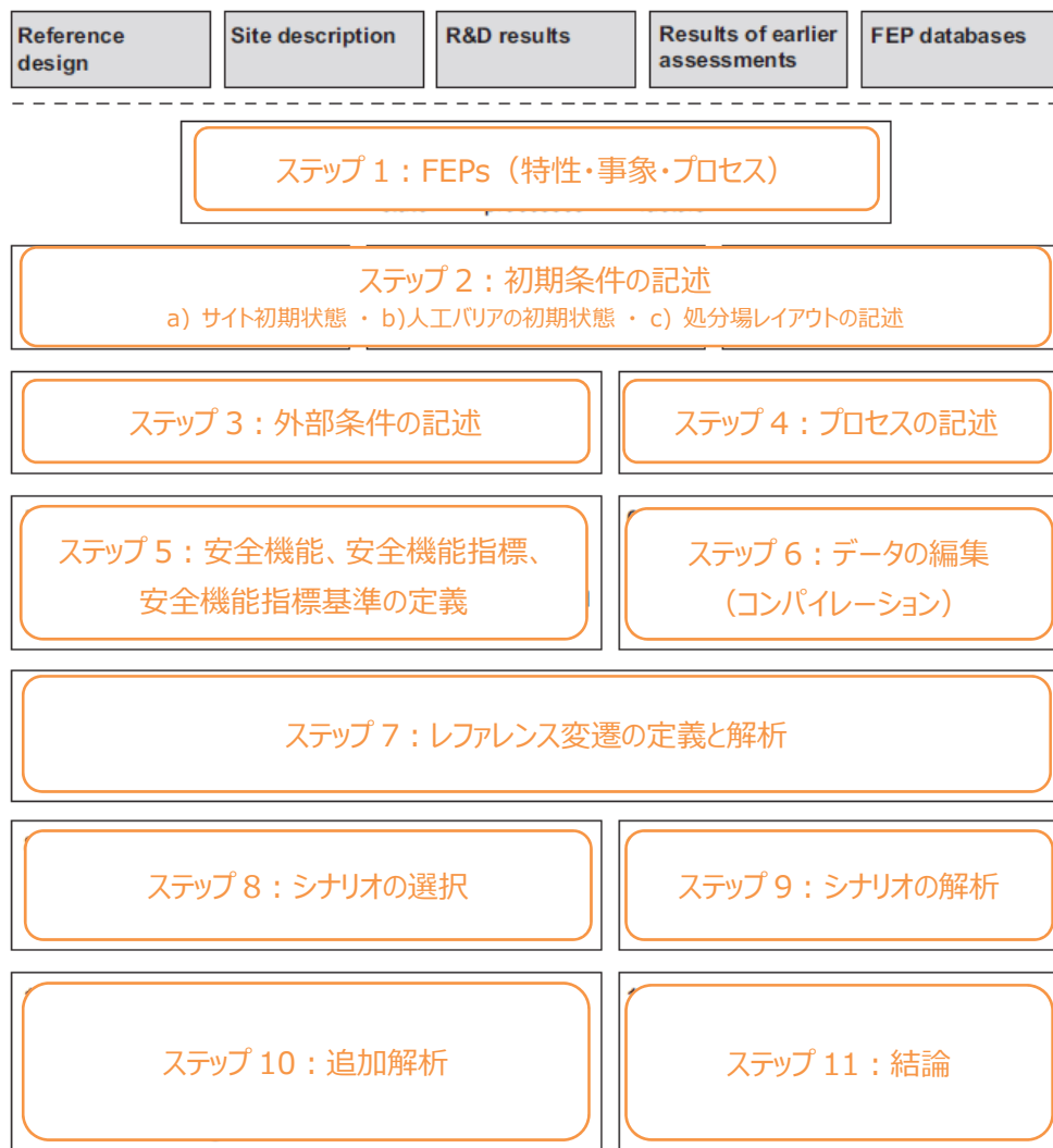
Figure 2-2. An outline of the eleven main steps of the SR-Site safety assessment. The boxes at the top above the dashed line are inputs to the assessment. The products of each step are described in detail in the main text. Together, the eleven steps represent the box “Safety assessment” in Figure 1-4.
