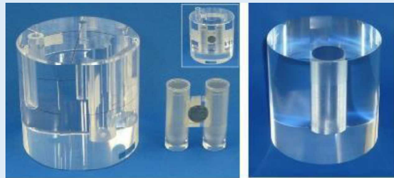
ORINSファントム Ref. ORINS-19 Thyroid radioiodine uptake measurement (1959)
