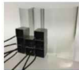
GAGG monitor (assembled 8 GAGG modules)
