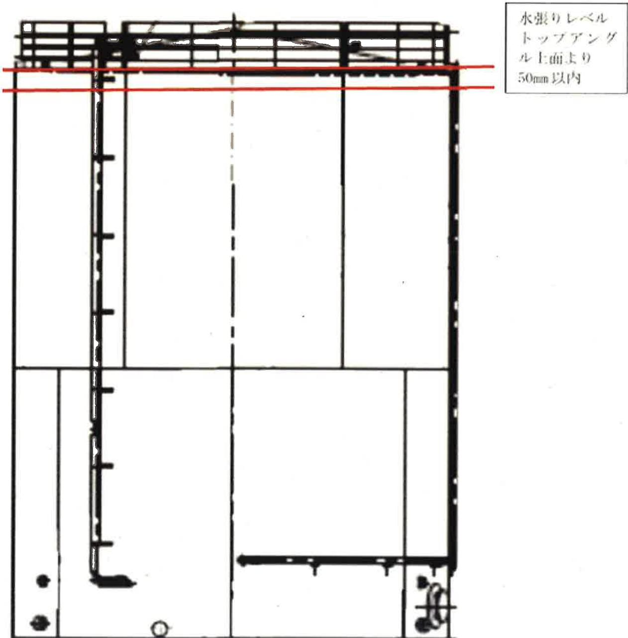
溶接型タンク概略図 (G 6) (1, 330m<sup>3</sup>)
