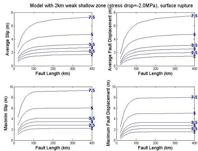
**Figure 11.** Models with weak shallow zone characterized with -2.0 MPa of stress drop: Average slip and maximum slip (left) and average fault displacement and maximum fault displacement (right) as a function of fault length for all the set of models. Each curve is indicated by a level of the corresponding dynamic stress drop at the end of each curve.
