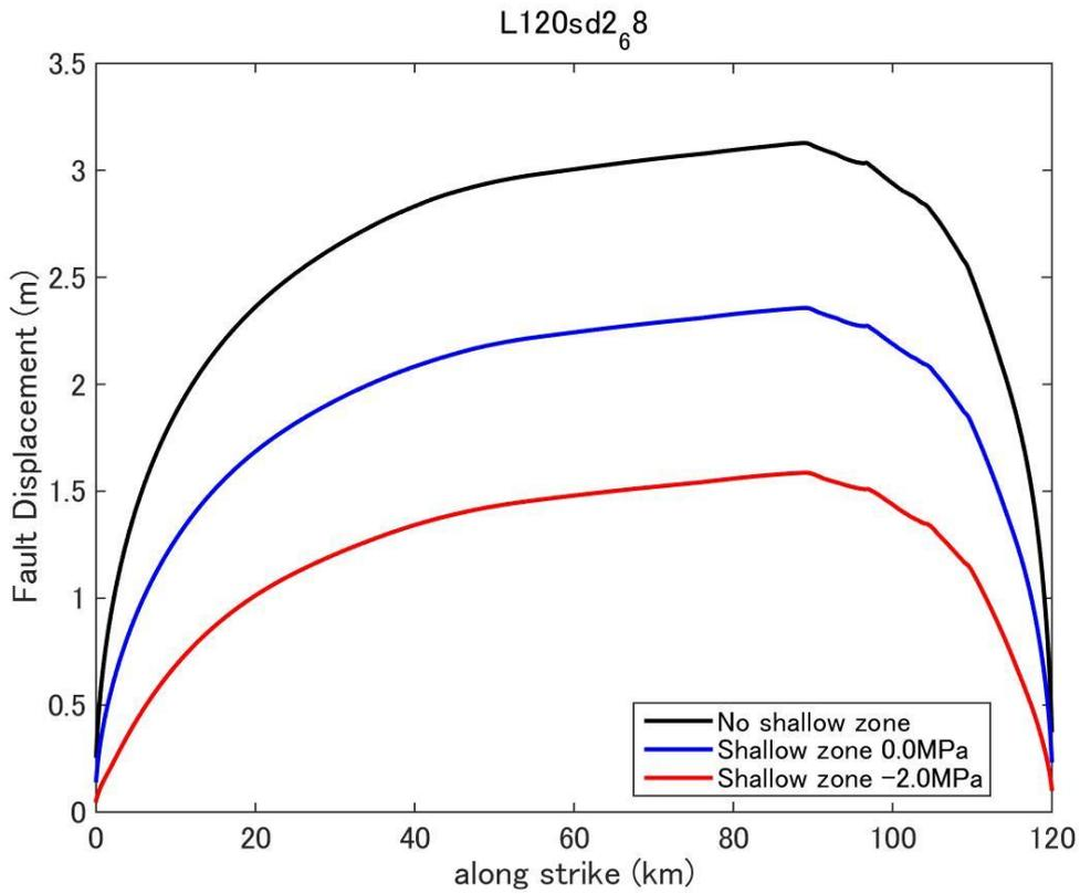
**Figure D31.** Fault displacement (surface rupture slip) distribution predicted by dynamic rupture model for a fault with fault length 120km and stress drop 2.0MPa.
