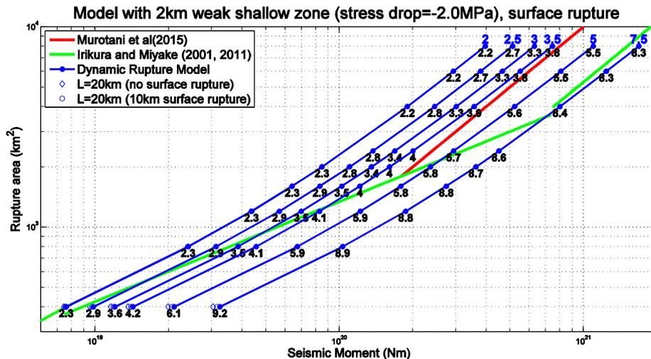
**Figure 14.** Models with weak shallow zone characterized with -2.0 MPa of stress drop:: Rupture area vs seismic moment for all the dynamic stress drop models and empirical models of Murotani et al (2015) and Irikura and Miyake (2001, 2011). The blue level at the end of each curve is the corresponding dynamic stress drop. The black number at each point is the static stress drop corresponding to each individual model.
