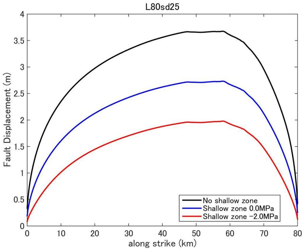
**Figure D22.** Fault displacement (surface rupture slip) distribution predicted by dynamic rupture model for a fault with fault length 80km and stress drop 2.5MPa.
