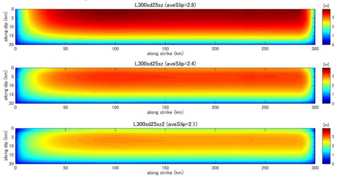
**Figure C46.** Final slip distribution predicted by dynamic rupture model for a fault with fault length 300km and stress drop 2.5MPa.
