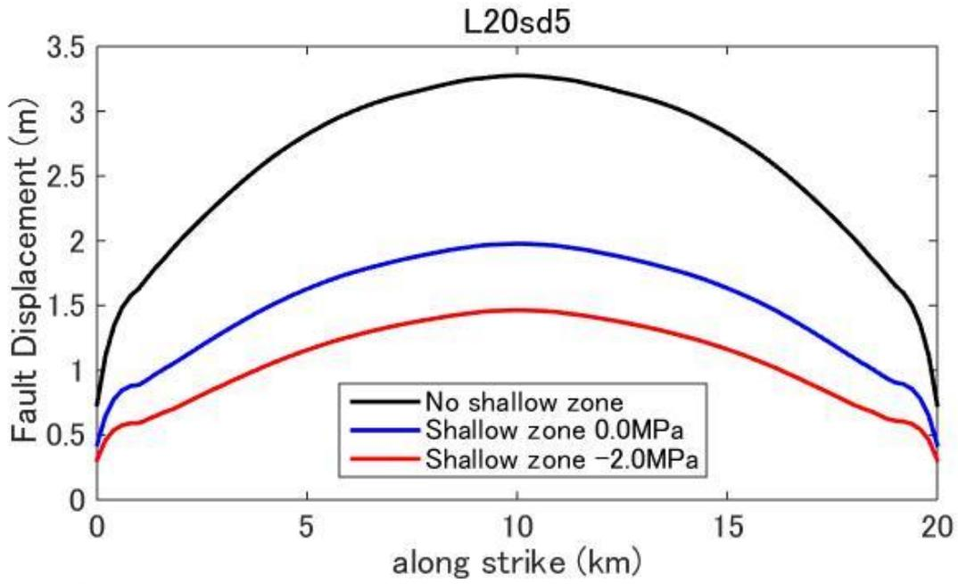
**Figure D3.** Fault displacement (surface rupture slip) distribution predicted by dynamic rupture model for a fault with fault length 20km and stress drop 5.0MPa.
