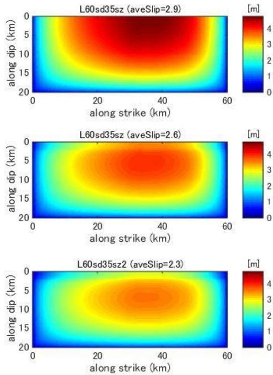
**Figure C17.** Final slip distribution predicted by dynamic rupture model for a fault with fault length 60km and stress drop 3.5MPa.
