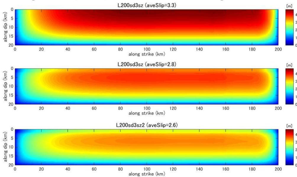
**Figure C38.** Final slip distribution predicted by dynamic rupture model for a fault with fault length 200km and stress drop 3.0MPa.
