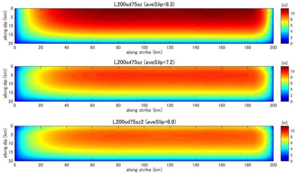
**Figure C42.** Final slip distribution predicted by dynamic rupture model for a fault with fault length 200km and stress drop 7.5MPa.
