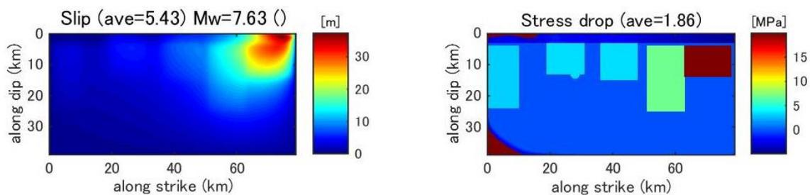
**Figure B1.** Slip distribution (left) from the dynamic asperity model (Masp1) that correspond to the stress drop distribution (right).
