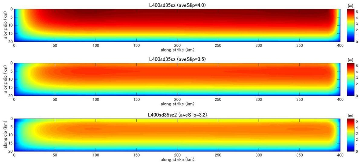
**Figure C53.** Final slip distribution predicted by dynamic rupture model for a fault with fault length 400km and stress drop 3.5MPa.
