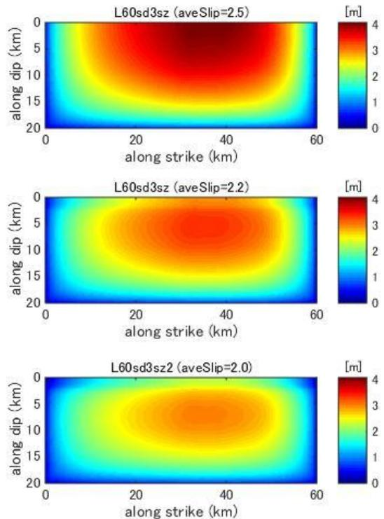
**Figure C14.** Final slip distribution predicted by dynamic rupture model for a fault with fault length 60km and stress drop 3.0MPa.
