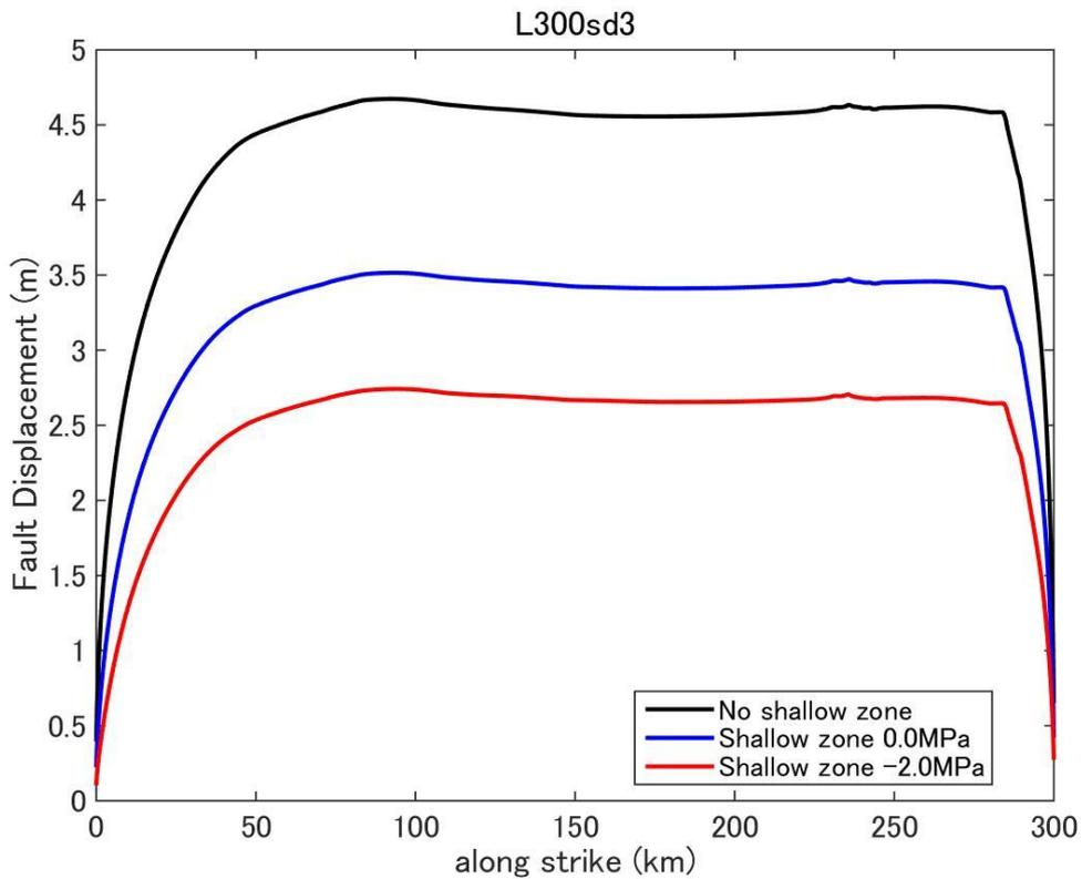
**Figure D44.** Fault displacement (surface rupture slip) distribution predicted by dynamic rupture model for a fault with fault length 300km and stress drop 3.0MPa.
