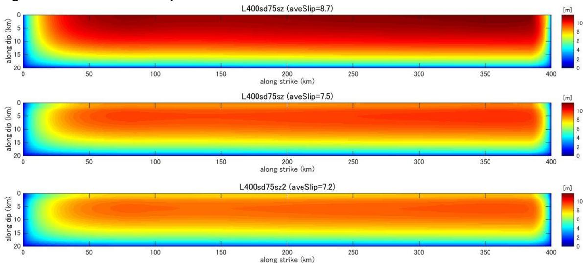
**Figure C54.** Final slip distribution predicted by dynamic rupture model for a fault with fault length 400km and stress drop 7.5MPa.
