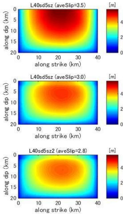
**Figure C9.** Final slip distribution predicted by dynamic rupture model for a fault with fault length 40km and stress drop 5.0MPa.
