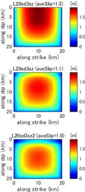
**Figure C2.** Final slip distribution predicted by dynamic rupture model for a fault with fault length 20km and stress drop 3.0MPa.
