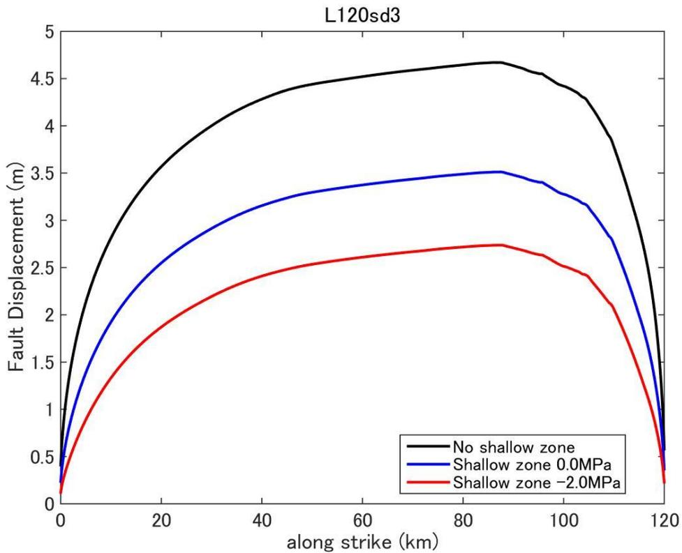
**Figure D32.** Fault displacement (surface rupture slip) distribution predicted by dynamic rupture model for a fault with fault length 120km and stress drop 3.0MPa.
