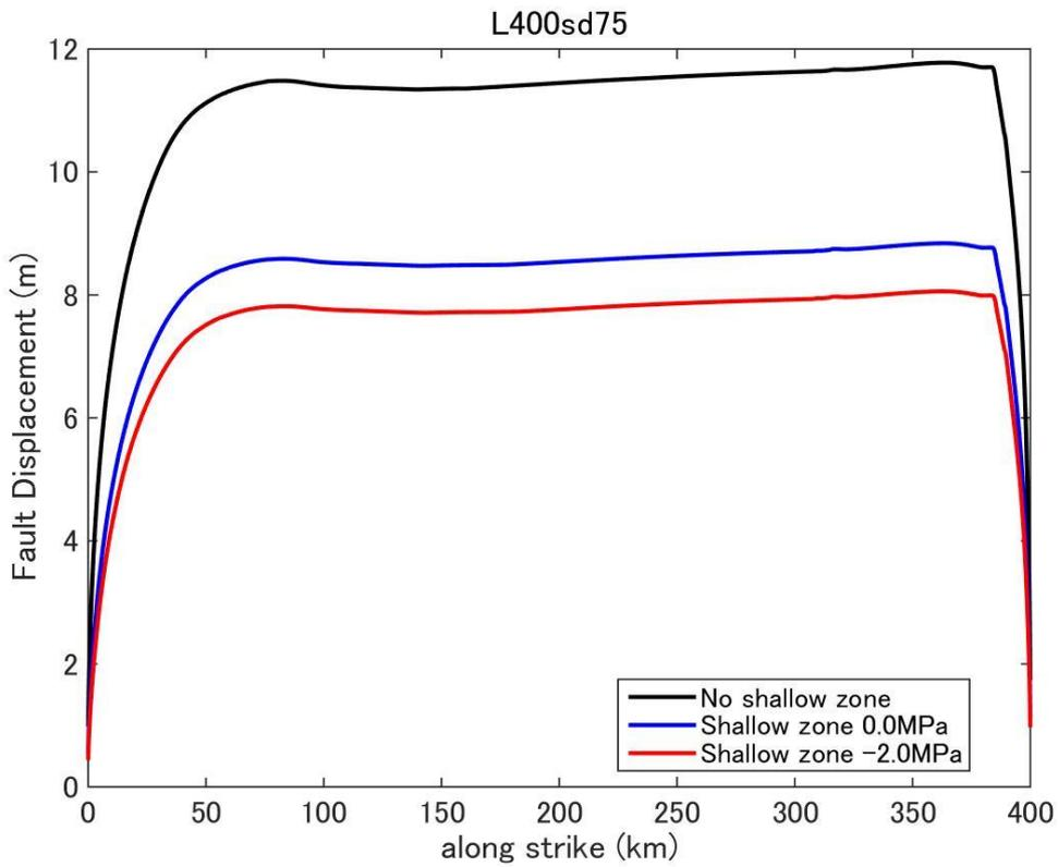
**Figure D54.** Fault displacement (surface rupture slip) distribution predicted by dynamic rupture model for a fault with fault length 400km and stress drop 7.5MPa.
