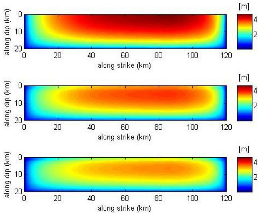
**Figure 7.** Final slip distribution predicted by dynamic rupture model for a fault with fault length 120km and stress drop 3.0MPa. [Top] no shallow zone model; [middle] weak shallow zone stress drop 0.0MPa; [bottom] weak shallow zone stress drop -2.0MPa.
