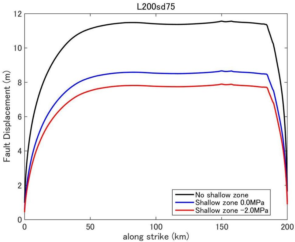
**Figure D42.** Fault displacement (surface rupture slip) distribution predicted by dynamic rupture model for a fault with fault length 200km and stress drop 7.5MPa.
