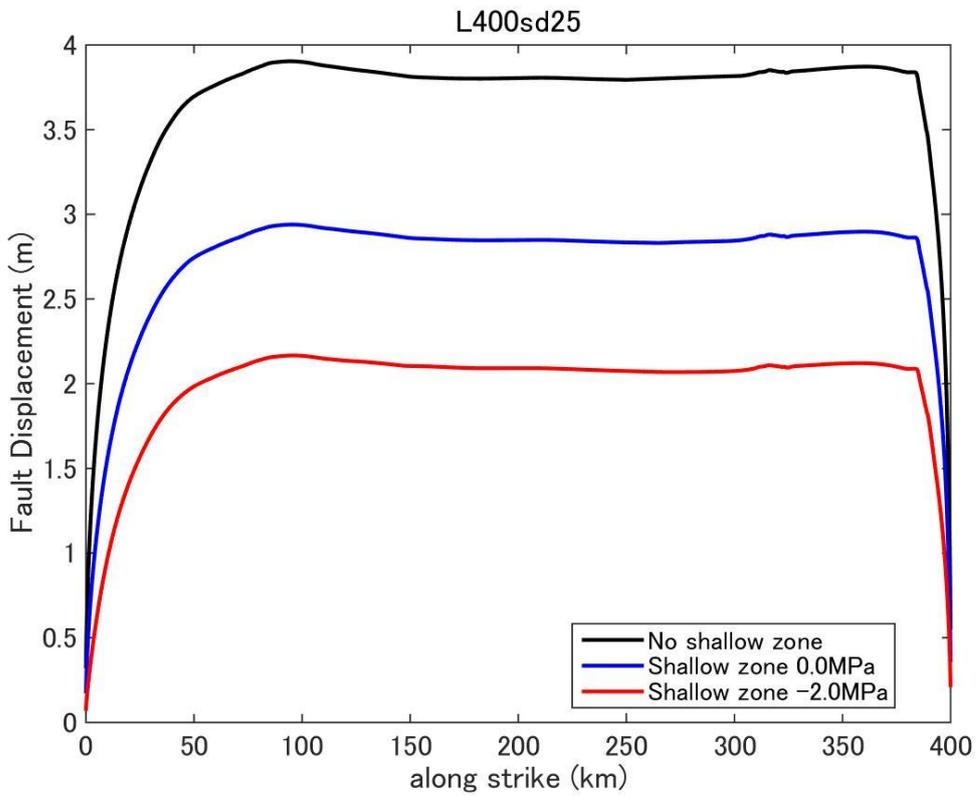
**Figure D52.** Fault displacement (surface rupture slip) distribution predicted by dynamic rupture model for a fault with fault length 400km and stress drop 2.5MPa.
