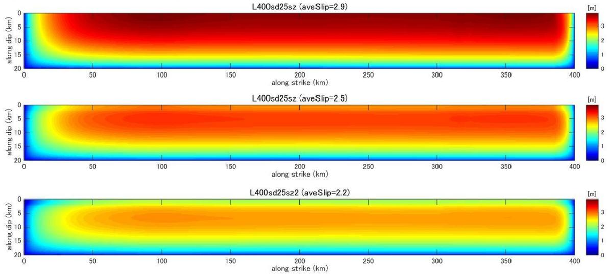
**Figure C52.** Final slip distribution predicted by dynamic rupture model for a fault with fault length 400km and stress drop 2.5MPa.
