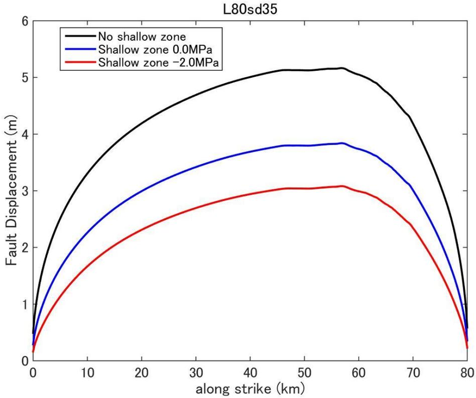
**Figure D23.** Fault displacement (surface rupture slip) distribution predicted by dynamic rupture model for a fault with fault length 80km and stress drop 3.5MPa.
