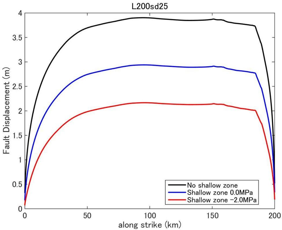
**Figure D40.** Fault displacement (surface rupture slip) distribution predicted by dynamic rupture model for a fault with fault length 200km and stress drop 2.5MPa.
