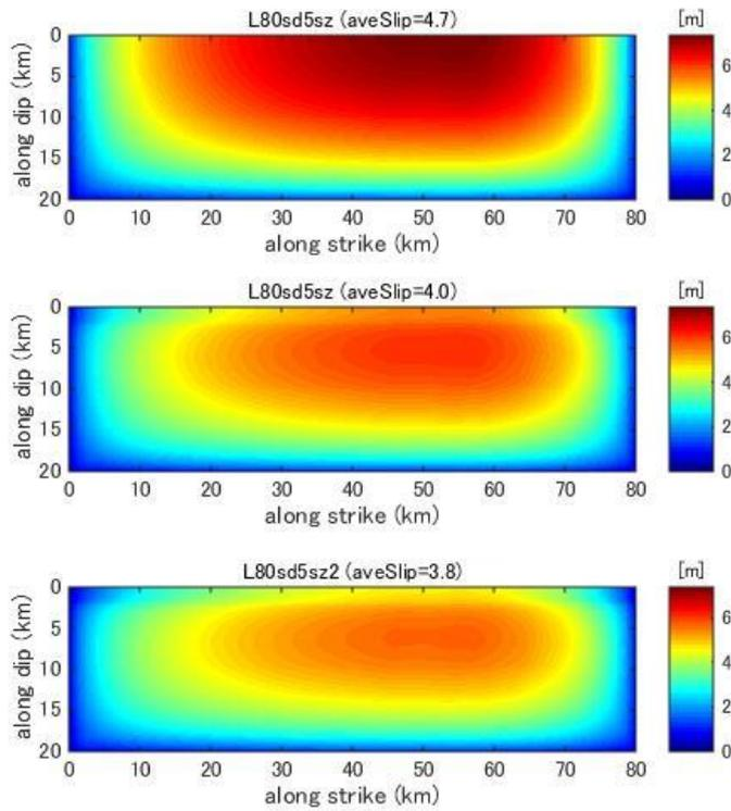
**Figure C21.** Final slip distribution predicted by dynamic rupture model for a fault with fault length 80km and stress drop 5.0MPa.
