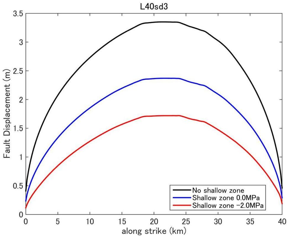
**Figure D8.** Fault displacement (surface rupture slip) distribution predicted by dynamic rupture model for a fault with fault length 40km and stress drop 3.0MPa.
