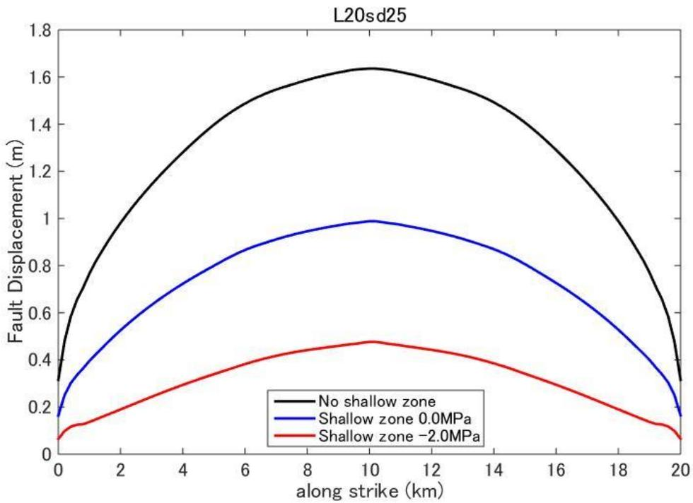
**Figure D4.** Fault displacement (surface rupture slip) distribution predicted by dynamic rupture model for a fault with fault length 20km and stress drop 2.5MPa.
