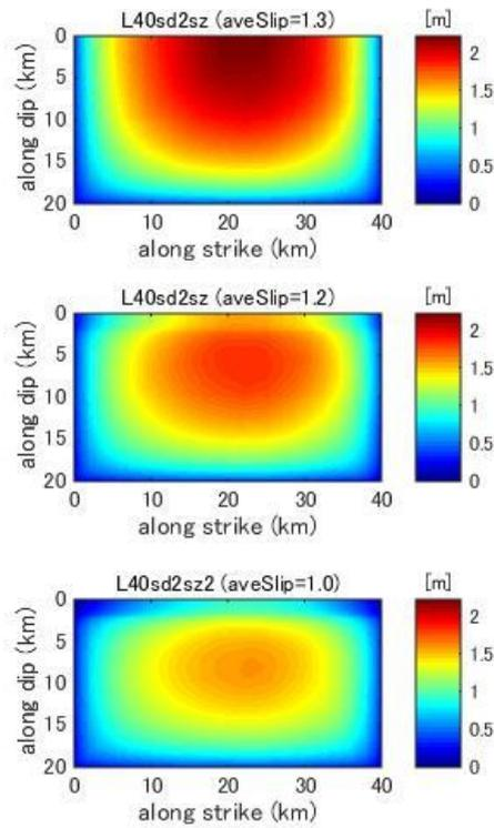
**Figure C7.** Final slip distribution predicted by dynamic rupture model for a fault with fault length 40km and stress drop 2.0MPa. [Top] no shallow zone model; [middle] weak shallow zone stress drop 0.0MPa; [bottom] weak shallow zone stress drop -2.0MPa.
