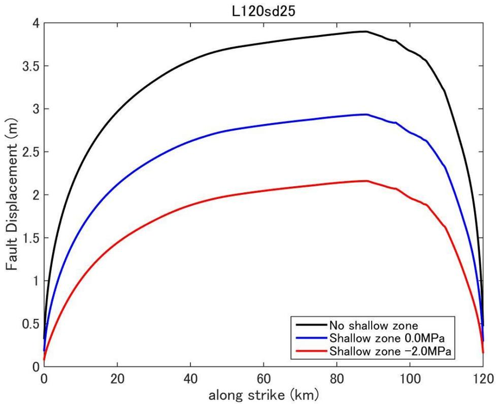
**Figure D34.** Fault displacement (surface rupture slip) distribution predicted by dynamic rupture model for a fault with fault length 120km and stress drop 2.5MPa.
