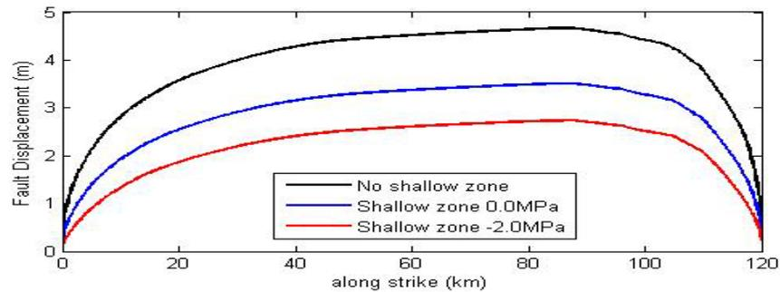
**Figure 8.** Fault displacement (surface rupture slip) distribution predicted by dynamic rupture
