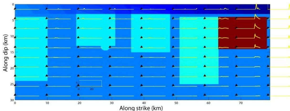
**Figure 4.** Slip velocity functions resulted from the dynamic rupture simulation of Masp8 model at selected points on the fault. These slip velocity waveforms are low pass filtered with a frequency cut of 3.0Hz.
