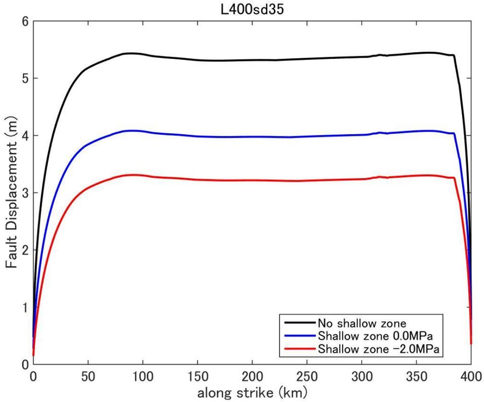
**Figure D53.** Fault displacement (surface rupture slip) distribution predicted by dynamic rupture model for a fault with fault length 400km and stress drop 3.5MPa.
