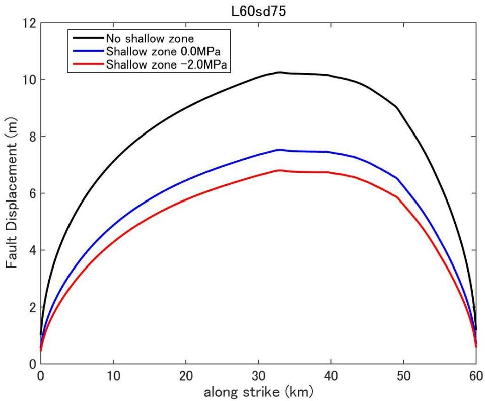
**Figure D18.** Fault displacement (surface rupture slip) distribution predicted by dynamic rupture model for a fault with fault length 60km and stress drop 7.5MPa.
