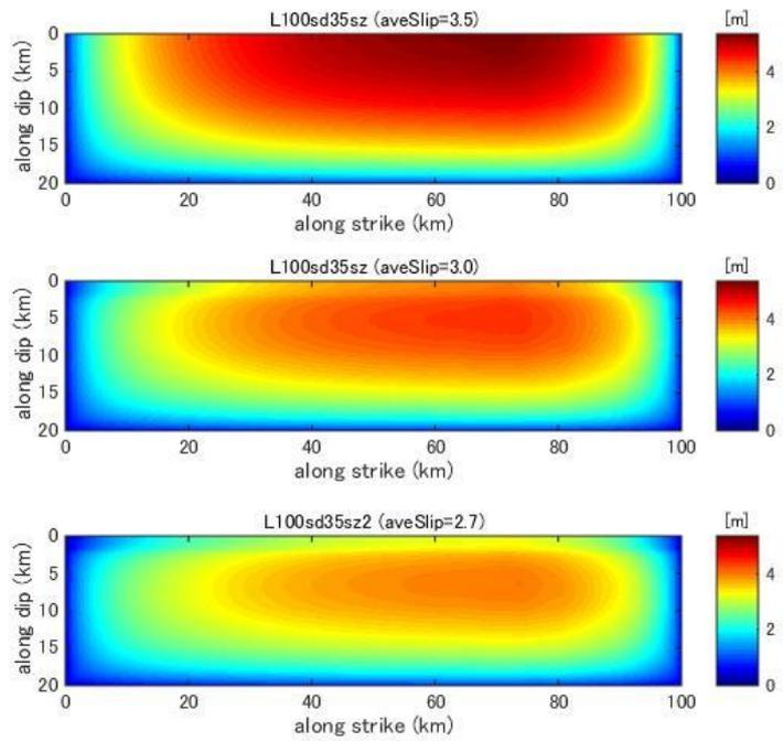
**Figure C29.** Final slip distribution predicted by dynamic rupture model for a fault with fault length 100km and stress drop 3.5MPa.
