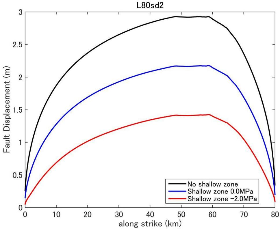
**Figure D19.** Fault displacement (surface rupture slip) distribution predicted by dynamic rupture model for a fault with fault length 80km and stress drop 2.0MPa.
