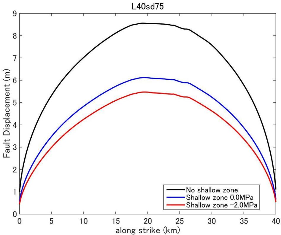
**Figure D12.** Fault displacement (surface rupture slip) distribution predicted by dynamic rupture model for a fault with fault length 40km and stress drop 7.5MPa.
