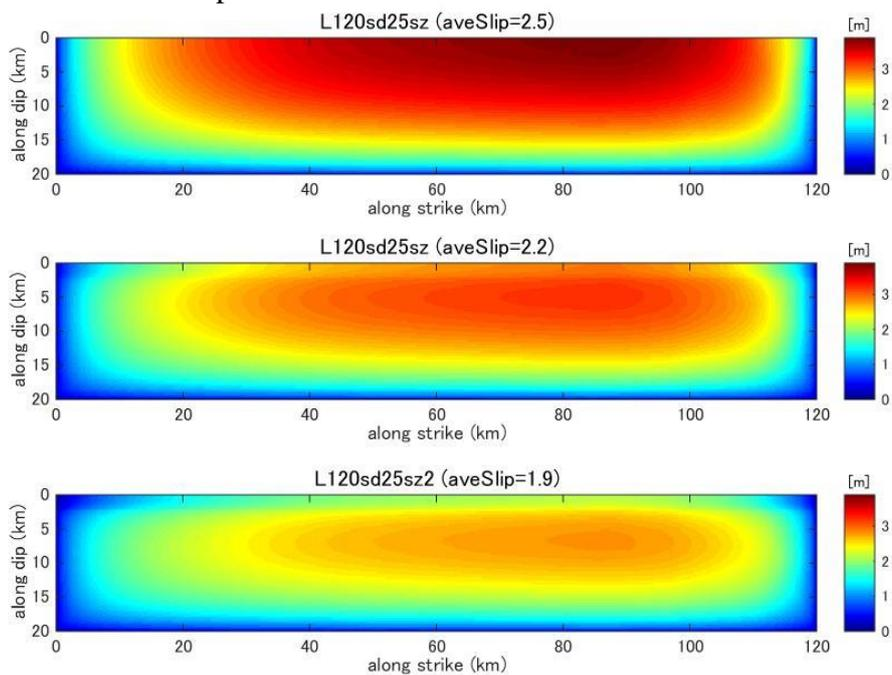
**Figure C34** Final slip distribution predicted by dynamic rupture model for a fault with fault length 120km and stress drop 2.5MPa.
