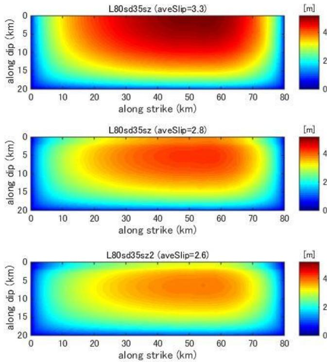
**Figure C23.** Final slip distribution predicted by dynamic rupture model for a fault with fault length 80km and stress drop 3.5MPa.
