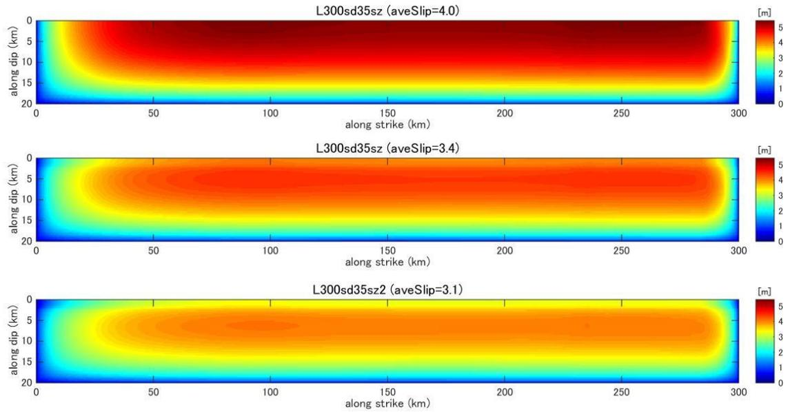
**Figure C47.** Final slip distribution predicted by dynamic rupture model for a fault with fault length 300km and stress drop 3.5MPa.
