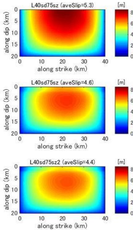
**Figure C12.** Final slip distribution predicted by dynamic rupture model for a fault with fault length 40km and stress drop 7.5MPa.
