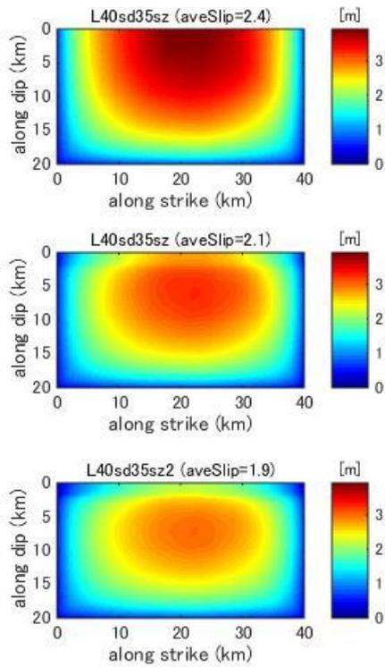
**Figure C11.** Final slip distribution predicted by dynamic rupture model for a fault with fault length 40km and stress drop 3.5MPa.
