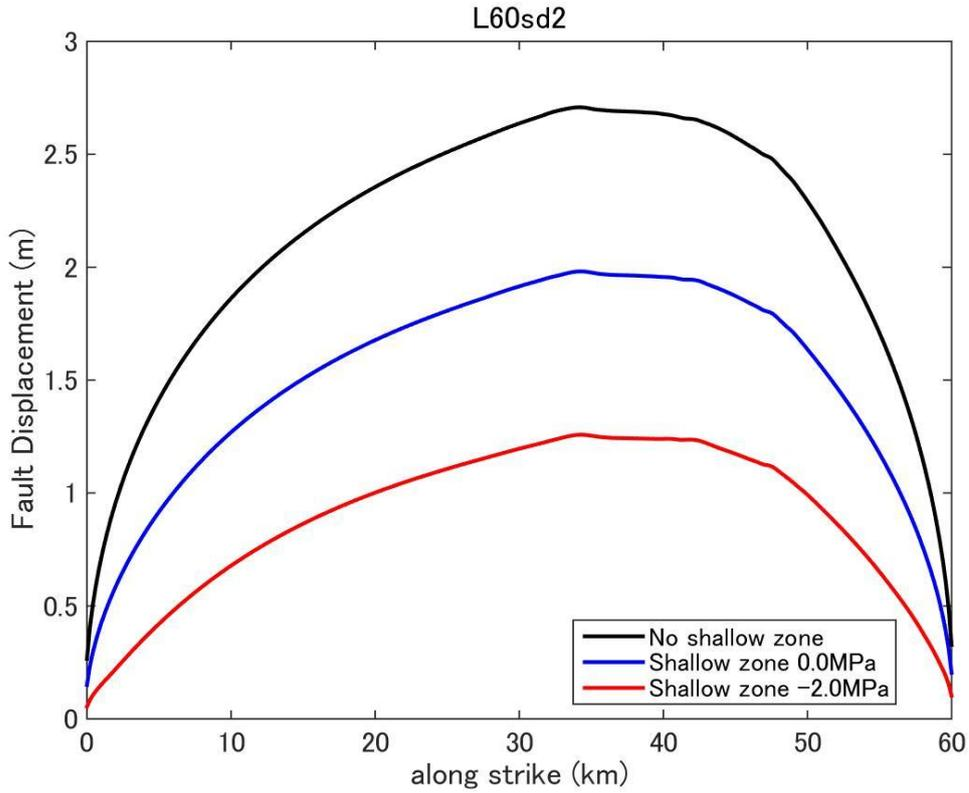
**Figure D13.** Fault displacement (surface rupture slip) distribution predicted by dynamic rupture model for a fault with fault length 60km and stress drop 2.0MPa.
