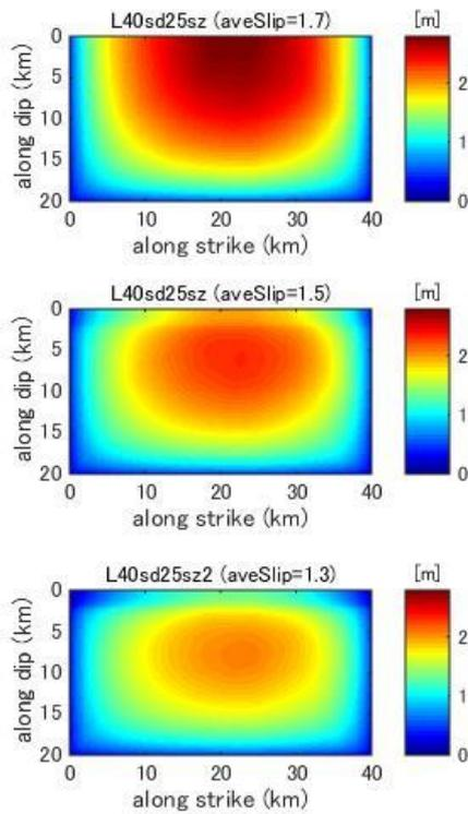
**Figure C10.** Final slip distribution predicted by dynamic rupture model for a fault with fault length 40km and stress drop 2.5MPa.
