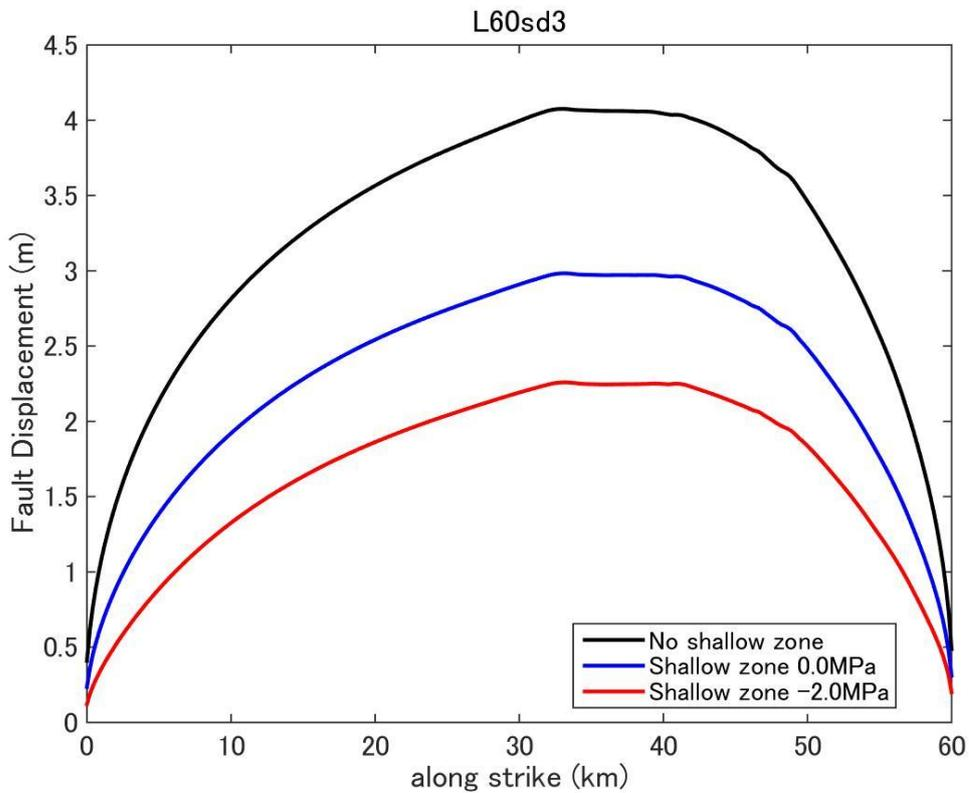
**Figure D14.** Fault displacement (surface rupture slip) distribution predicted by dynamic rupture model for a fault with fault length 60km and stress drop 3.0MPa.
