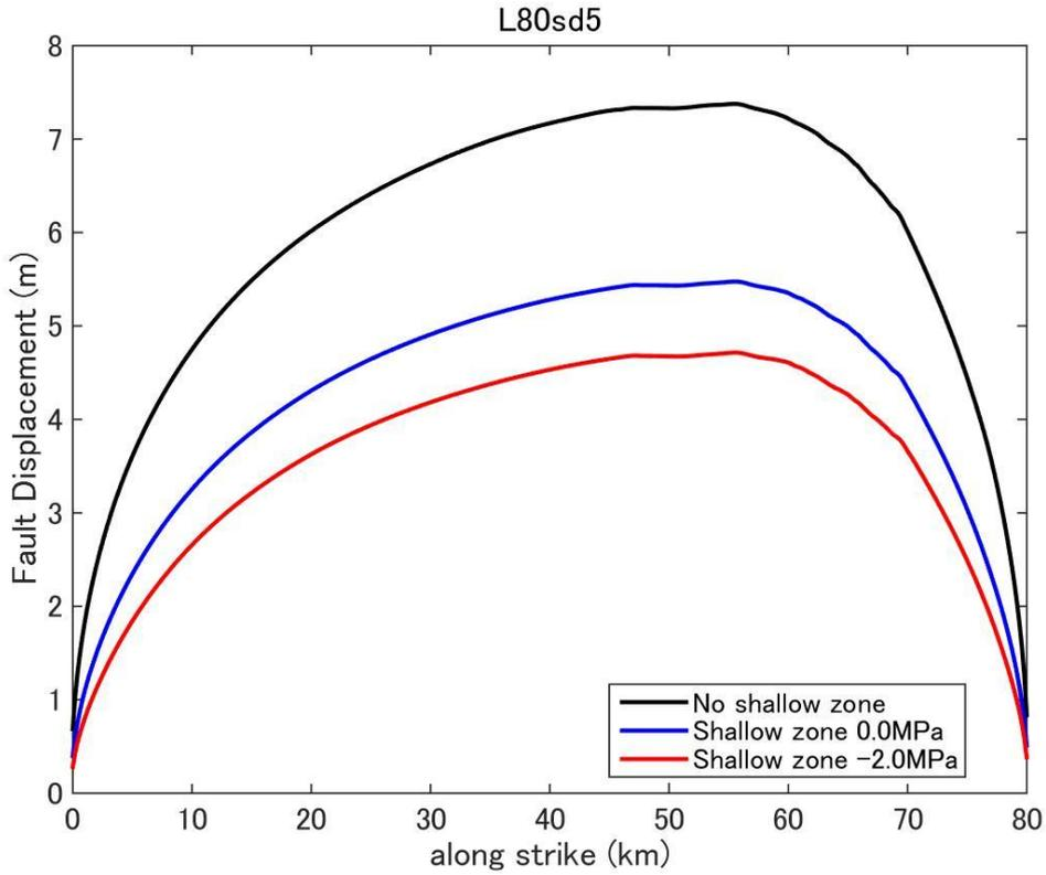
**Figure D21.** Fault displacement (surface rupture slip) distribution predicted by dynamic rupture model for a fault with fault length 80km and stress drop 5.0MPa.
