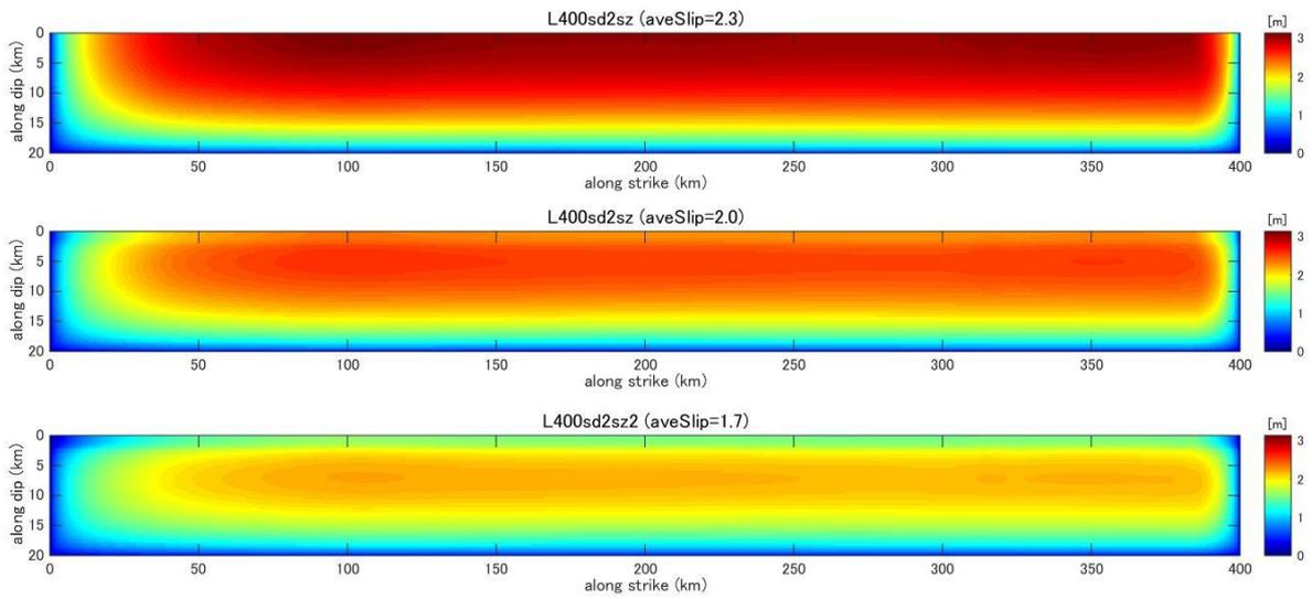
**Figure C49.** Final slip distribution predicted by dynamic rupture model for a fault with fault length 400km and stress drop 2.0MPa. [Top] no shallow zone model; [middle] weak shallow zone stress drop 0.0MPa; [bottom] weak shallow zone stress drop -2.0MPa.
