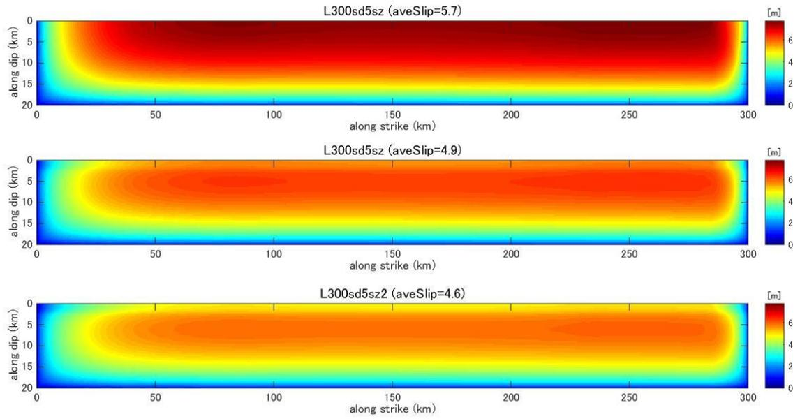
**Figure C45.** Final slip distribution predicted by dynamic rupture model for a fault with fault length 300km and stress drop 5.0MPa.
