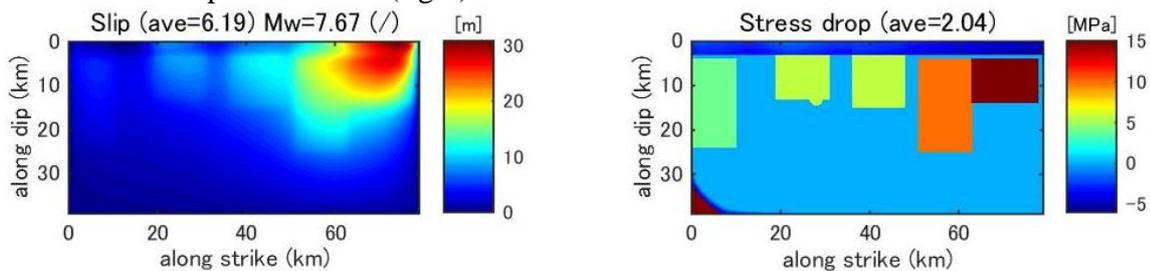
**Figure B2.** Slip distribution (left) from the dynamic asperity model (Masp2) that correspond to the stress drop distribution (right).
