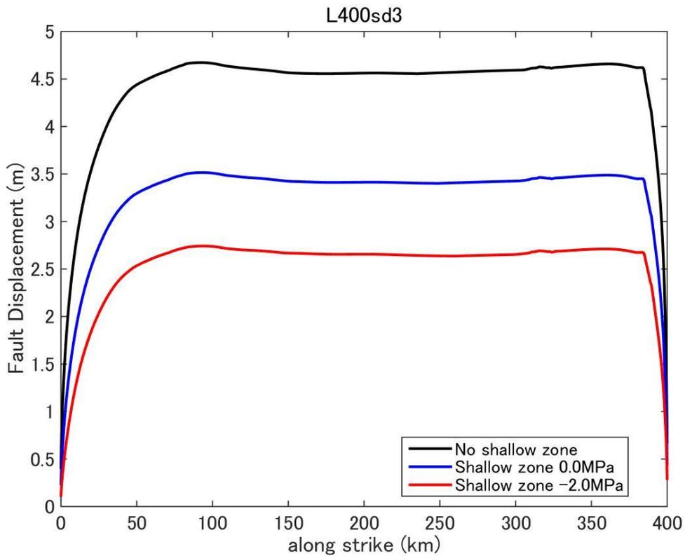
**Figure D50.** Fault displacement (surface rupture slip) distribution predicted by dynamic rupture model for a fault with fault length 400km and stress drop 3.0MPa.
