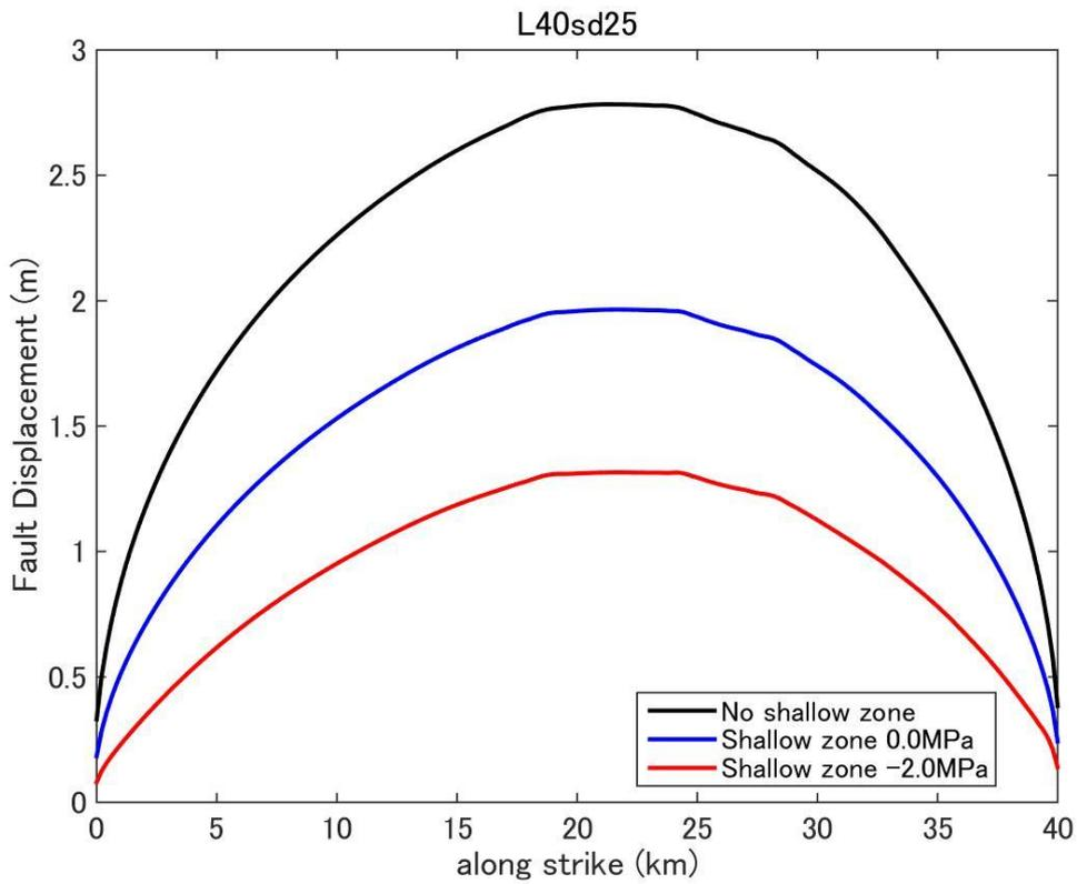
**Figure D10.** Fault displacement (surface rupture slip) distribution predicted by dynamic rupture model for a fault with fault length 40km and stress drop 2.5MPa.
