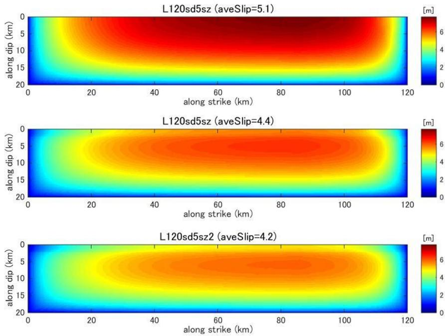
**Figure C33.** Final slip distribution predicted by dynamic rupture model for a fault with fault length 120km and stress drop 5.0MPa.
