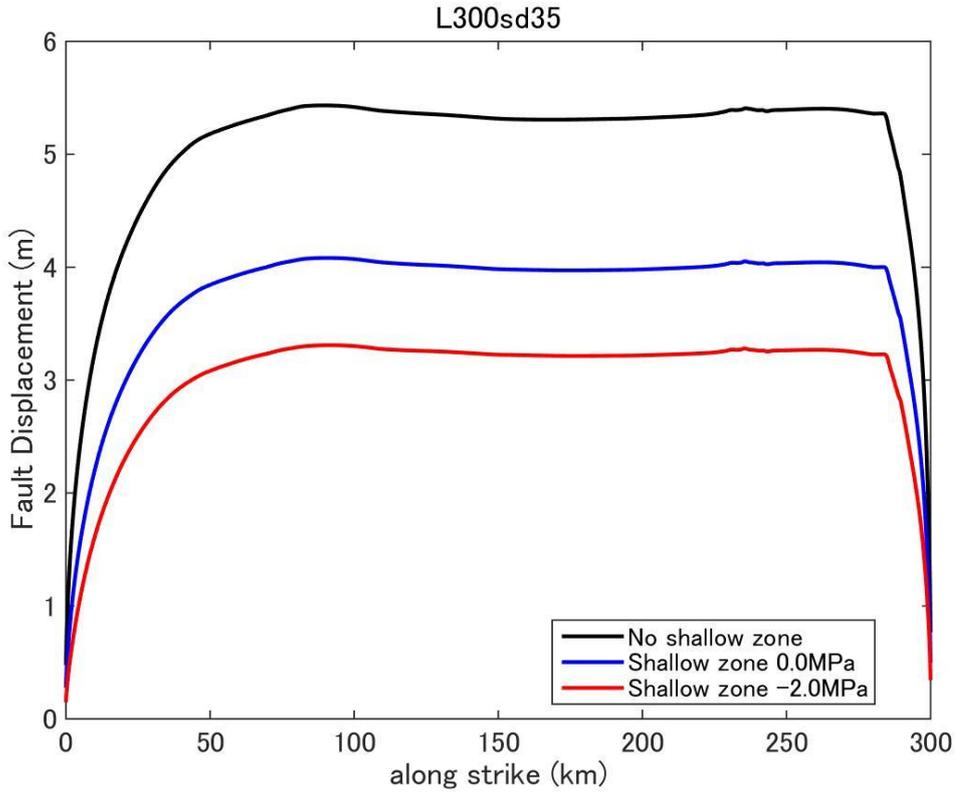
**Figure D47.** Fault displacement (surface rupture slip) distribution predicted by dynamic rupture model for a fault with fault length 300km and stress drop 3.5MPa.
