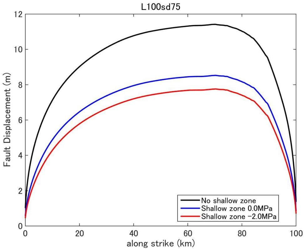
**Figure D30.** Fault displacement (surface rupture slip) distribution predicted by dynamic rupture model for a fault with fault length 100km and stress drop 7.5MPa.
