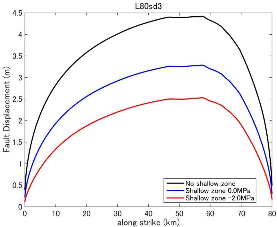
**Figure D20.** Fault displacement (surface rupture slip) distribution predicted by dynamic rupture model for a fault with fault length 80km and stress drop 3.0MPa.
