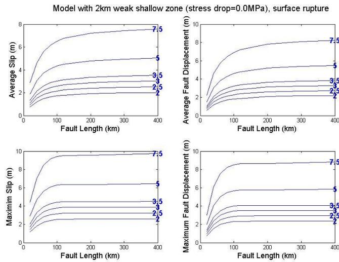
**Figure 10.** Models with weak shallow zone characterized with 0.0 MPa of stress drop: Average slip and maximum slip (left) and average fault displacement and maximum fault displacement (right) as a function of fault length for all the set of models. Each curve is indicated by a level of the corresponding dynamic stress drop at the end of each curve.
