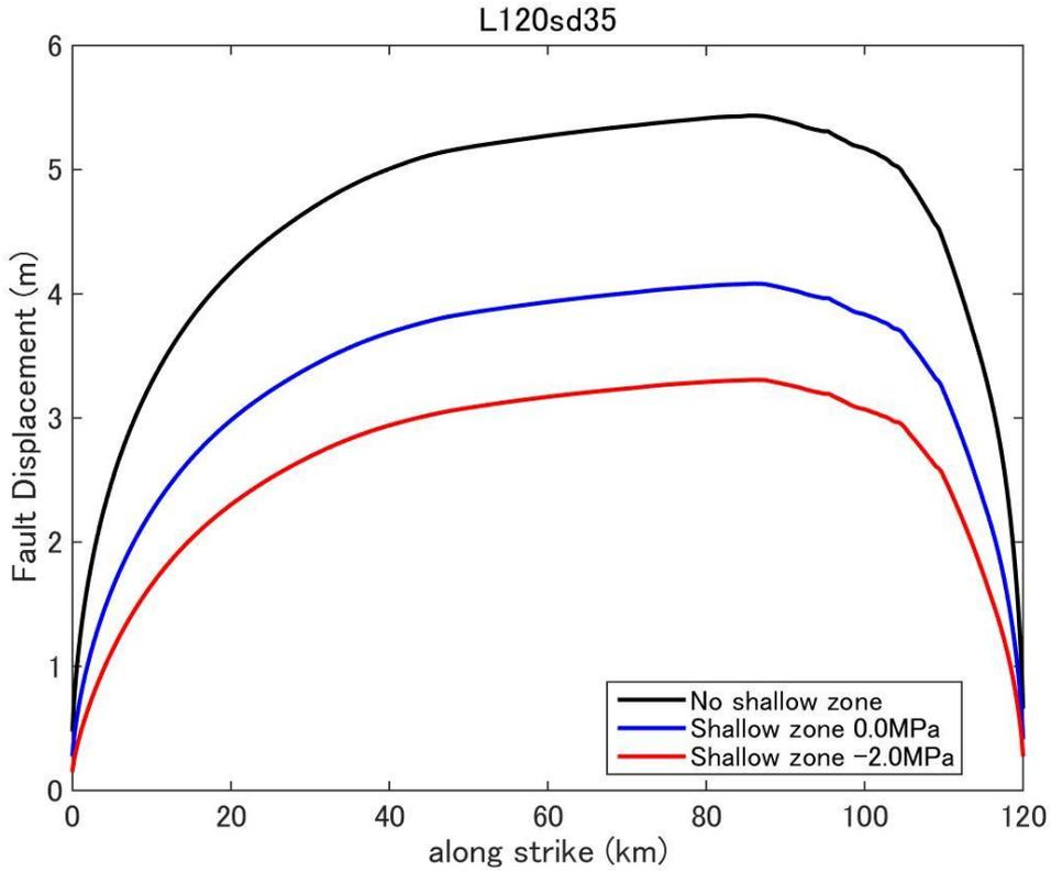
**Figure D35.** Fault displacement (surface rupture slip) distribution predicted by dynamic rupture model for a fault with fault length 120km and stress drop 3.5MPa.
