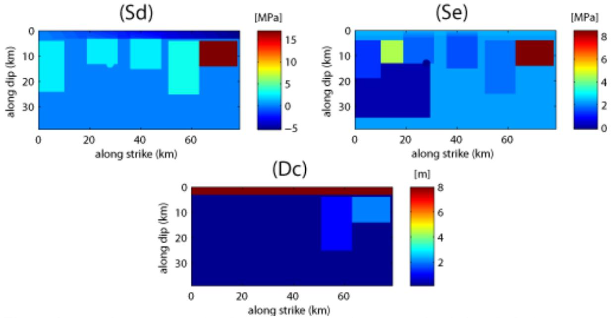
**Figure 2.** Asperity source model (Masp8) for dynamic rupture simulation. Left shows stress drop distribution, right strength excess and bottom critical slip distance (Dc)
