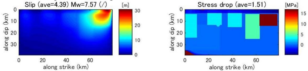
**Figure B7.** Slip distribution (left) from the dynamic asperity model (Masp7) that correspond to the stress drop distribution (right).
