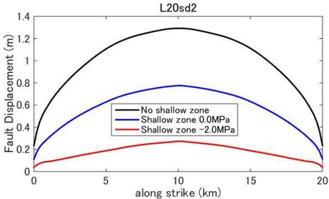
**Figure D1.** Fault displacement (surface rupture slip) distribution predicted by dynamic rupture model for a fault with fault length 20km and stress drop 2.0MPa.
