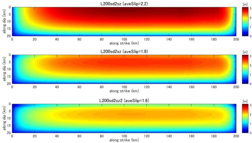
**Figure C37.** Final slip distribution predicted by dynamic rupture model for a fault with fault length 200km and stress drop 2.0MPa. [Top] no shallow zone model; [middle] weak shallow zone stress drop 0.0MPa; [bottom] weak shallow zone stress drop -2.0MPa.
