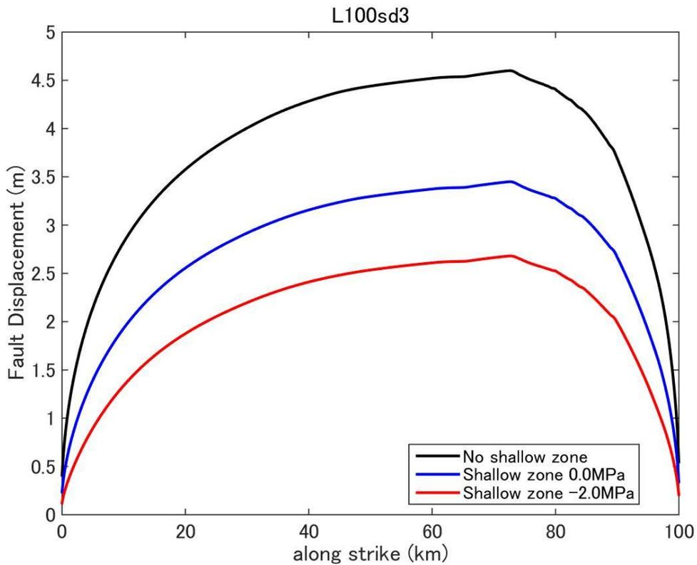
**Figure D26.** Fault displacement (surface rupture slip) distribution predicted by dynamic rupture model for a fault with fault length 100km and stress drop 3.0MPa.
