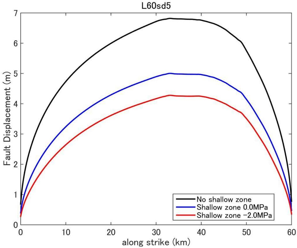
**Figure D15.** Fault displacement (surface rupture slip) distribution predicted by dynamic rupture model for a fault with fault length 60km and stress drop 5.0MPa.
