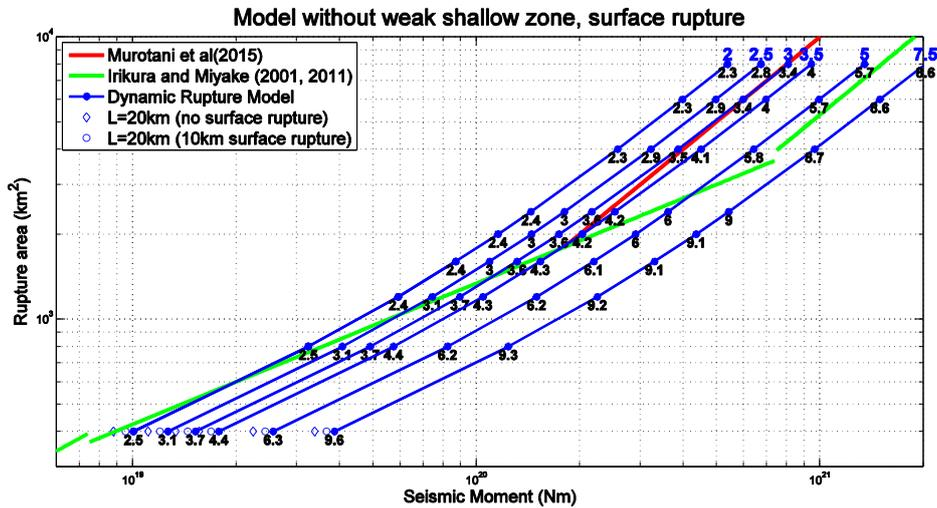
**Figure 12.** Models without weak shallow zone: Rupture area vs seismic moment for all the dynamic stress drop models and empirical models of Murotani et al (2015) and Irikura and Miyake (2001, 2011). The blue level at the end of each curve is the corresponding dynamic stress drop. The black number at each point is the static stress drop corresponding to each individual model.
