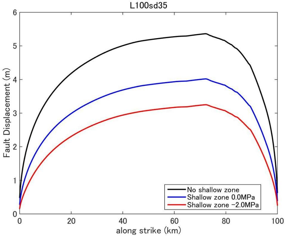
**Figure D29.** Fault displacement (surface rupture slip) distribution predicted by dynamic rupture model for a fault with fault length 100km and stress drop 3.5MPa.
