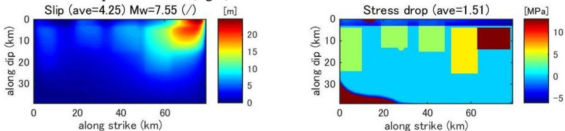
**Figure B3.** Slip distribution (left) from the dynamic asperity model (Masp3) that correspond to the stress drop distribution (right).
