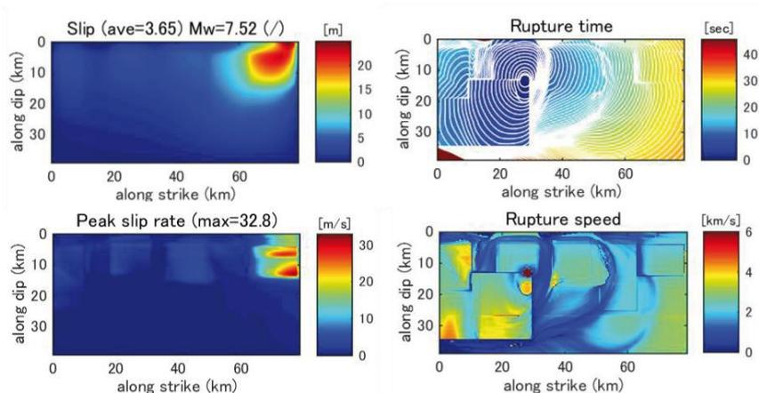
**Figure 3.** Dynamic rupture solution of Masp8 model represented by the final slip distribution (top left), peak slip velocity (bottom left), rupture time (top right) and rupture speed (bottom right). Contour lines on the rupture time images are also the rupture time each 0.5 seconds.
