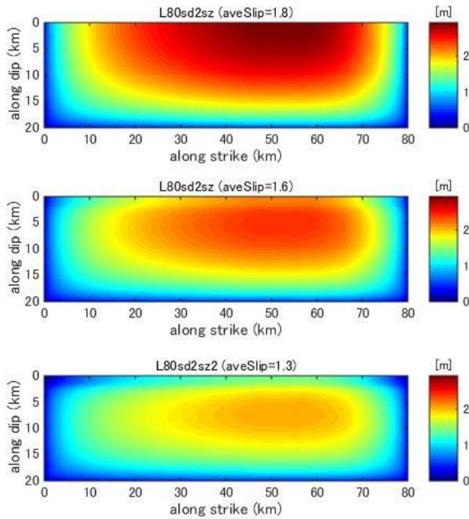
**Figure C19.** Final slip distribution predicted by dynamic rupture model for a fault with fault length 80km and stress drop 2.0MPa. [Top] no shallow zone model; [middle] weak shallow zone stress drop 0.0MPa; [bottom] weak shallow zone stress drop -2.0MPa.
