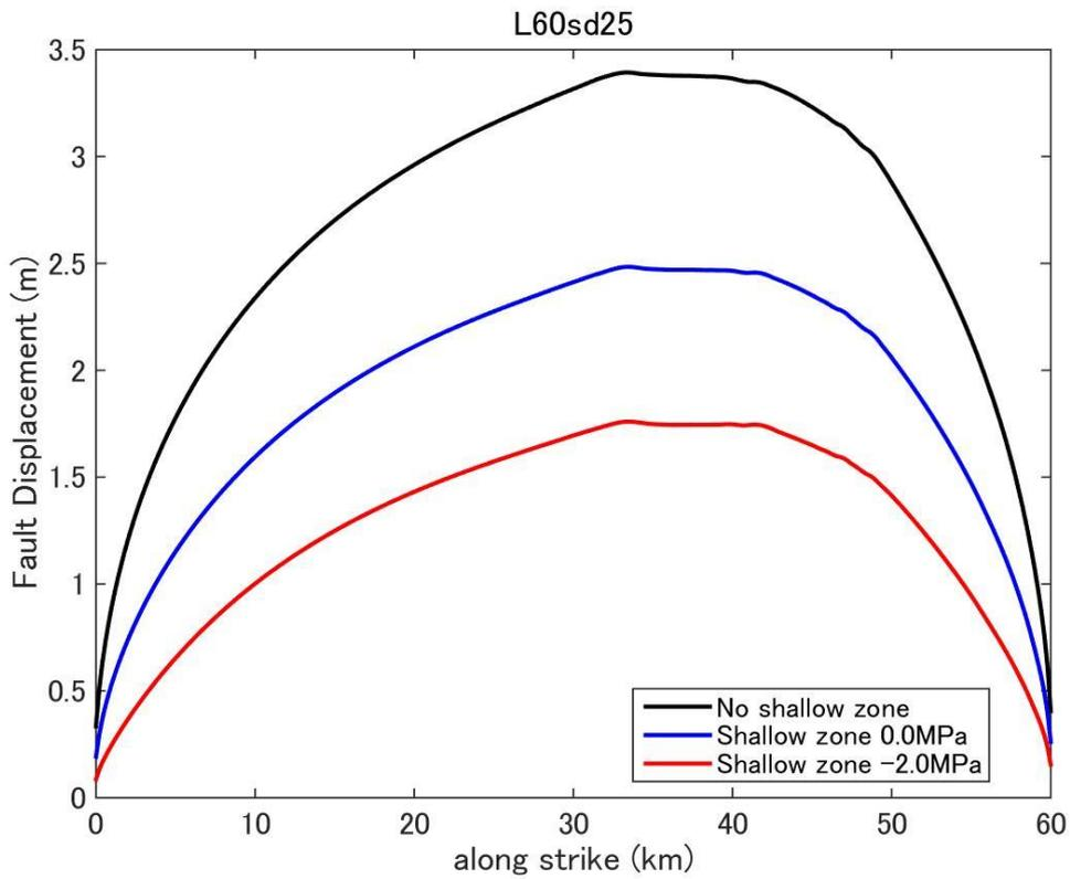
**Figure D16.** Fault displacement (surface rupture slip) distribution predicted by dynamic rupture model for a fault with fault length 60km and stress drop 2.5MPa.
