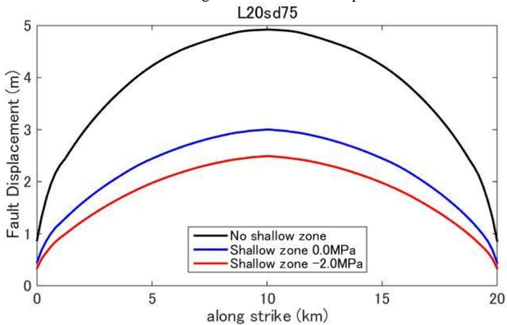
**Figure D6.** Fault displacement (surface rupture slip) distribution predicted by dynamic rupture model for a fault with fault length 20km and stress drop 7.5MPa.
