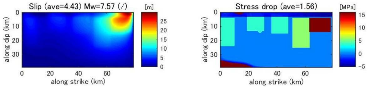
**Figure B5.** Slip distribution (left) from the dynamic asperity model (Masp5) that correspond to the stress drop distribution (right).
