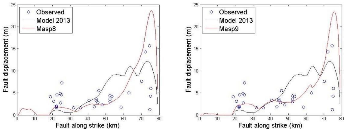
**Figure 6.** Fault displacement compared with observed data, [left] Masp8 model: [right] Masp9 Model. In both cases the results of the 2013 fiscal year is included as reference
