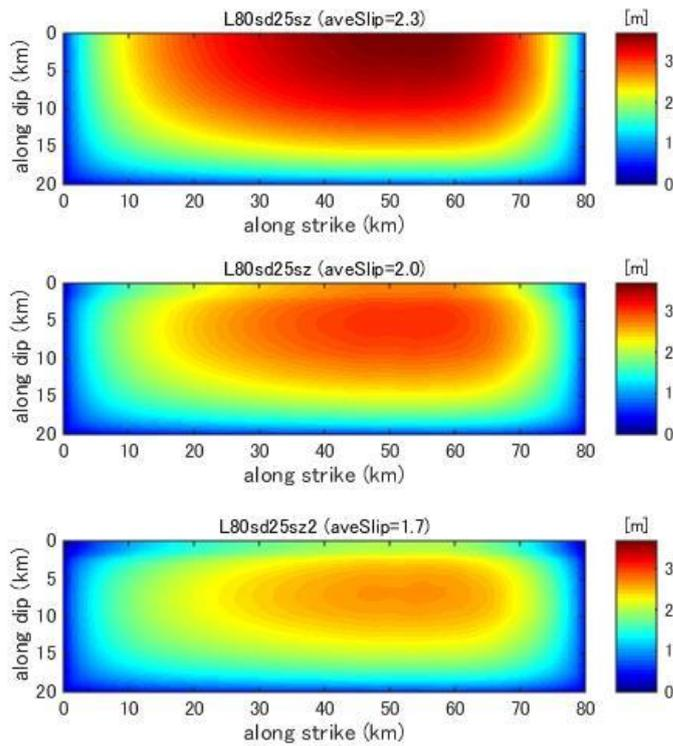
**Figure C22.** Final slip distribution predicted by dynamic rupture model for a fault with fault length 80km and stress drop 2.5MPa.
