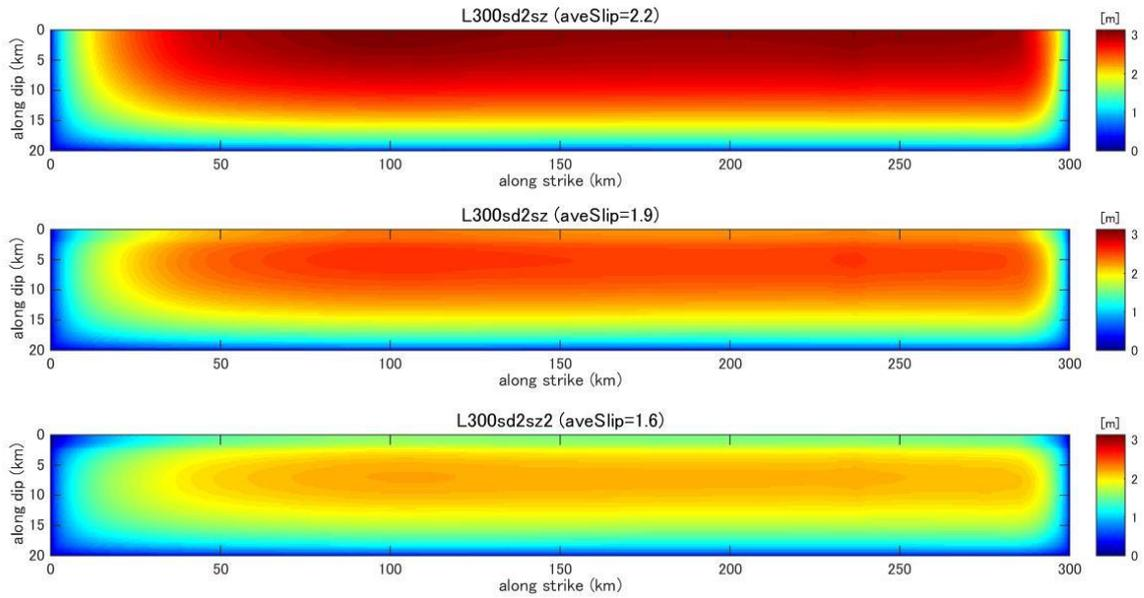
**Figure C43.** Final slip distribution predicted by dynamic rupture model for a fault with fault length 300km and stress drop 2.0MPa. [Top] no shallow zone model; [middle] weak shallow zone stress drop 0.0MPa; [bottom] weak shallow zone stress drop -2.0MPa.
