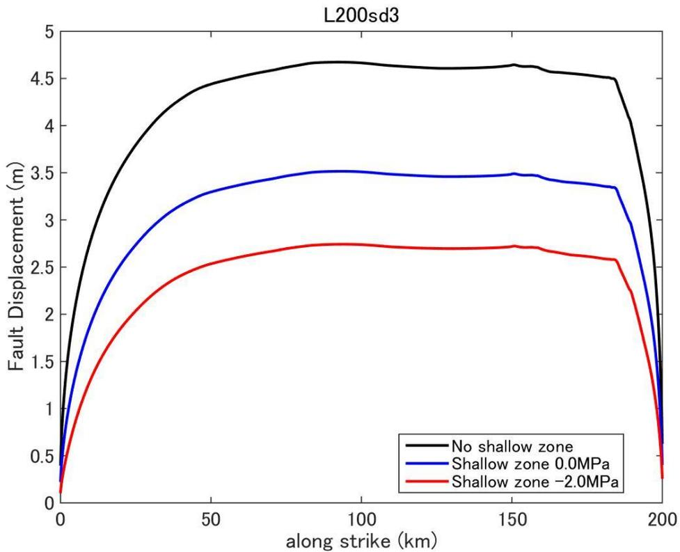
**Figure D38.** Fault displacement (surface rupture slip) distribution predicted by dynamic rupture model for a fault with fault length 200km and stress drop 3.0MPa.
