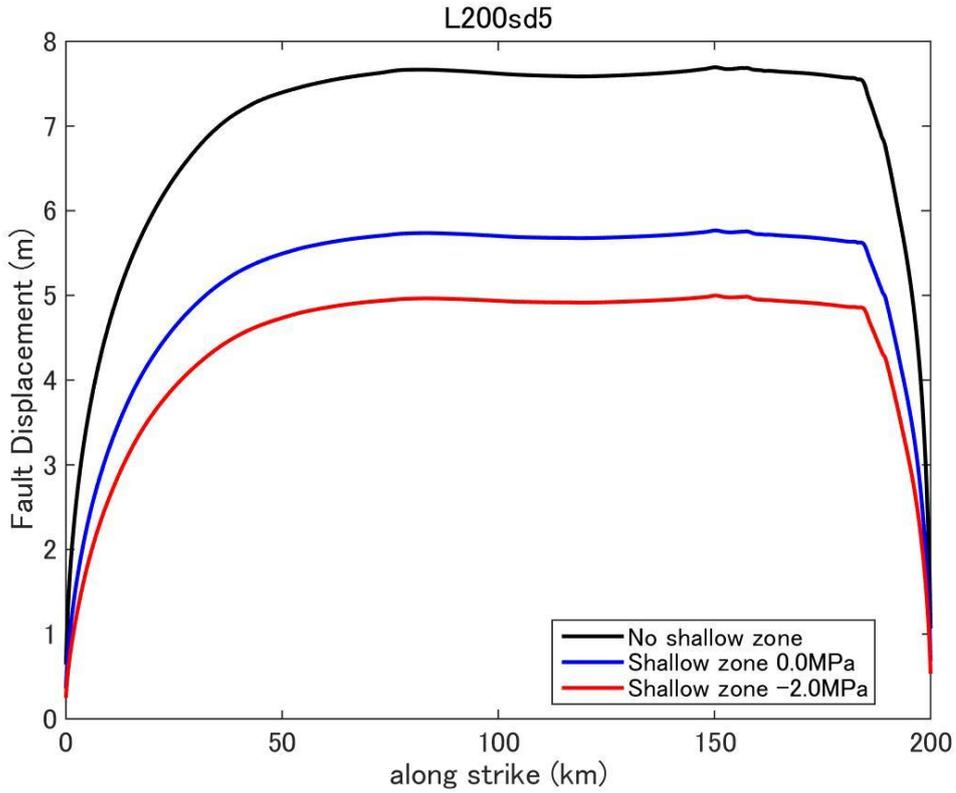
**Figure D39.** Fault displacement (surface rupture slip) distribution predicted by dynamic rupture model for a fault with fault length 200km and stress drop 5.0MPa.
