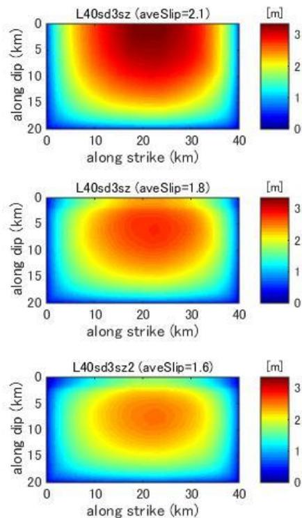
**Figure C8.** Final slip distribution predicted by dynamic rupture model for a fault with fault length 40km and stress drop 3.0MPa.
