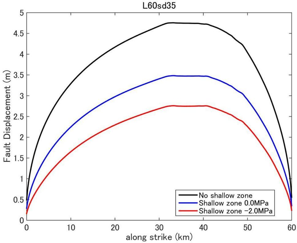
**Figure D17.** Fault displacement (surface rupture slip) distribution predicted by dynamic rupture model for a fault with fault length 60km and stress drop 3.5MPa.
