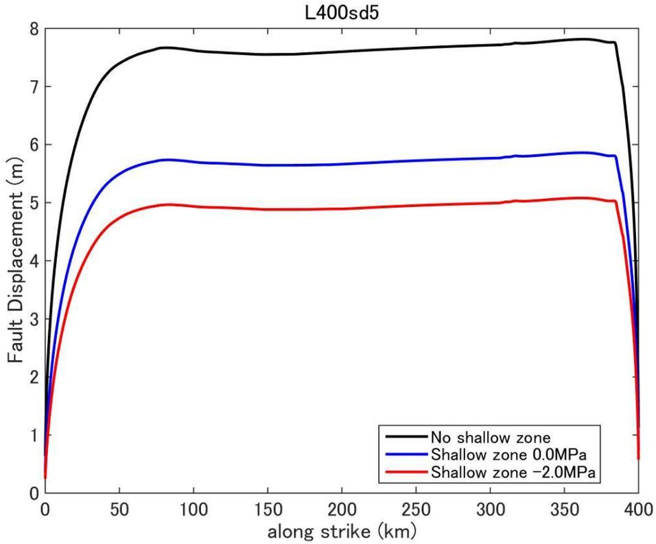
**Figure D51.** Fault displacement (surface rupture slip) distribution predicted by dynamic rupture model for a fault with fault length 400km and stress drop 5.0MPa.
