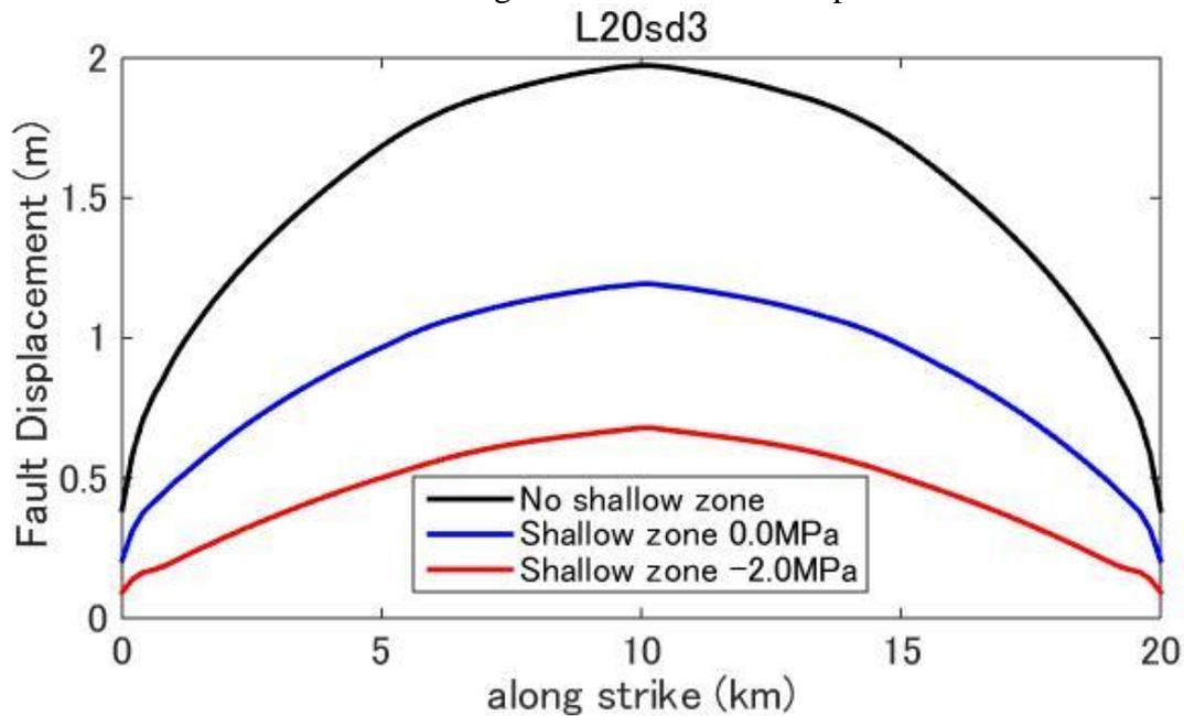
**Figure D2.** Fault displacement (surface rupture slip) distribution predicted by dynamic rupture model for a fault with fault length 20km and stress drop 3.0MPa.
