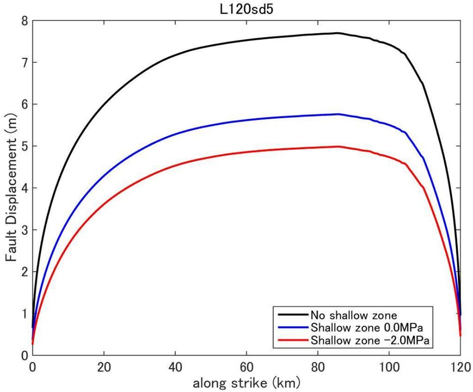
**Figure D33.** Fault displacement (surface rupture slip) distribution predicted by dynamic rupture model for a fault with fault length 120km and stress drop 5.0MPa.
