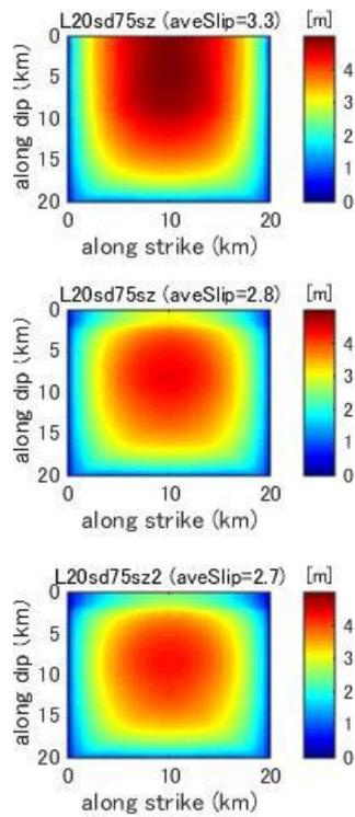
**Figure C6.** Final slip distribution predicted by dynamic rupture model for a fault with fault length 20km and stress drop 7.5MPa.
