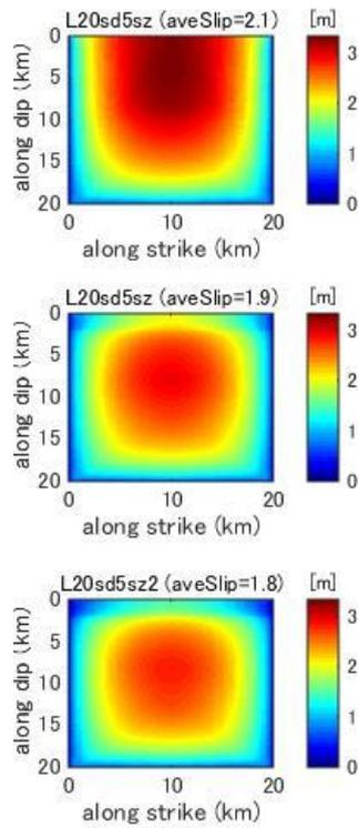
**Figure C3.** Final slip distribution predicted by dynamic rupture model for a fault with fault length 20km and stress drop 5.0MPa.
