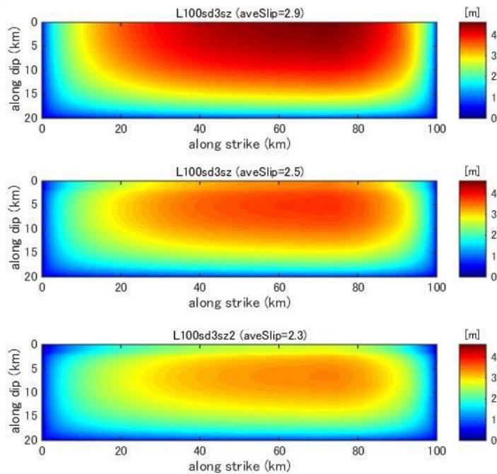
**Figure C26.** Final slip distribution predicted by dynamic rupture model for a fault with fault length 100km and stress drop 3.0MPa.
