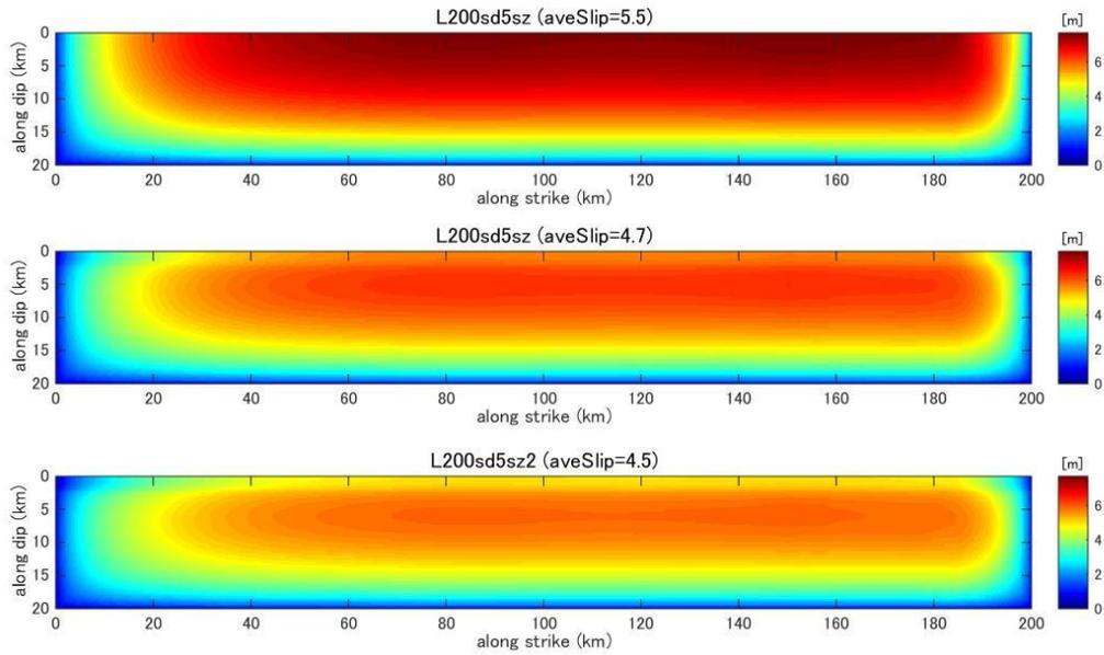
**Figure C39.** Final slip distribution predicted by dynamic rupture model for a fault with fault length 200km and stress drop 5.0MPa.
