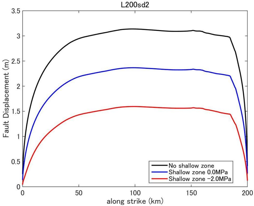
**Figure D37.** Fault displacement (surface rupture slip) distribution predicted by dynamic rupture model for a fault with fault length 200km and stress drop 2.0MPa.
