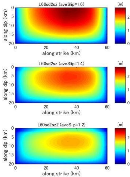
**Figure C13.** Final slip distribution predicted by dynamic rupture model for a fault with fault length 60km and stress drop 2.0MPa. [Top] no shallow zone model; [middle] weak shallow zone stress drop 0.0MPa; [bottom] weak shallow zone stress drop -2.0MPa.
