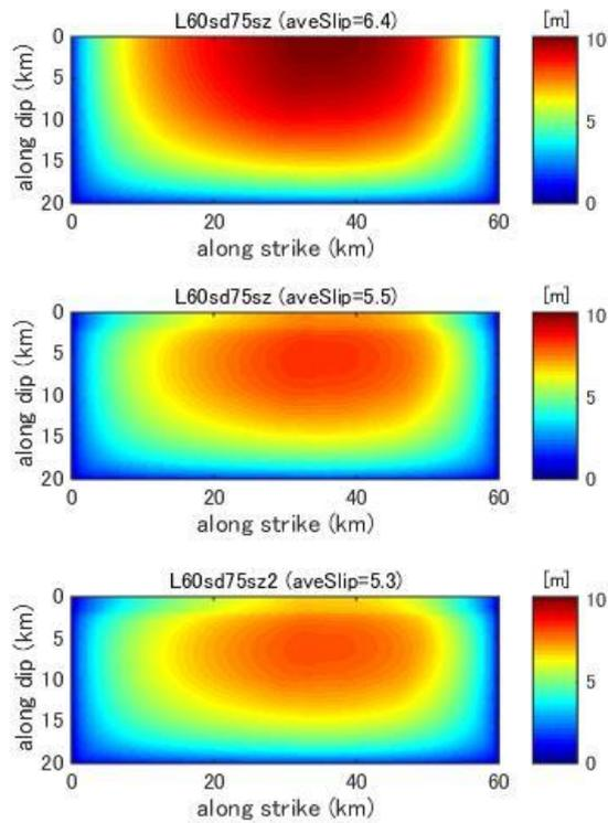
**Figure C18.** Final slip distribution predicted by dynamic rupture model for a fault with fault length 60km and stress drop 7.5MPa.
