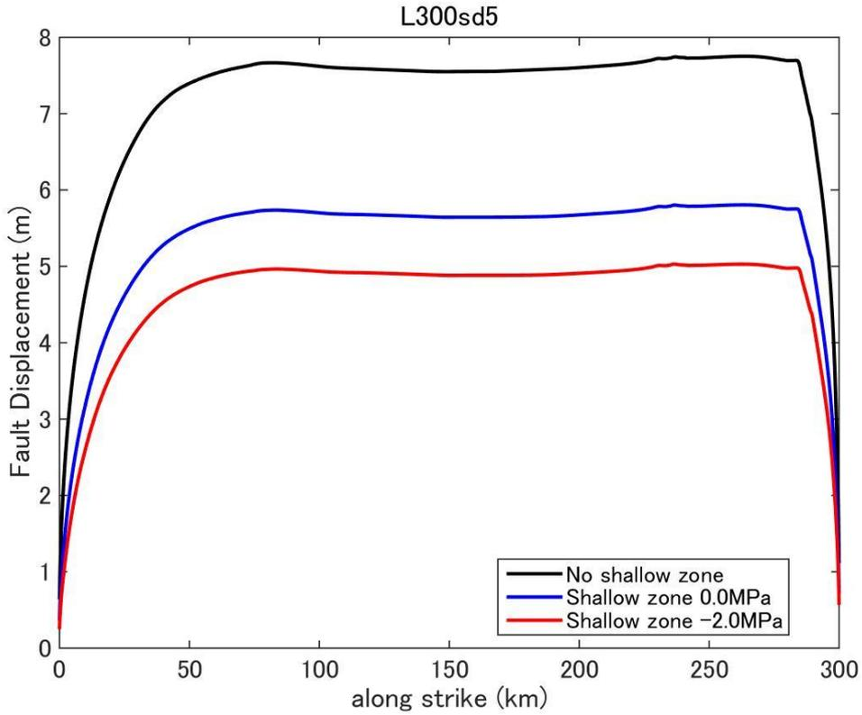
**Figure D45.** Fault displacement (surface rupture slip) distribution predicted by dynamic rupture model for a fault with fault length 300km and stress drop 5.0MPa.
