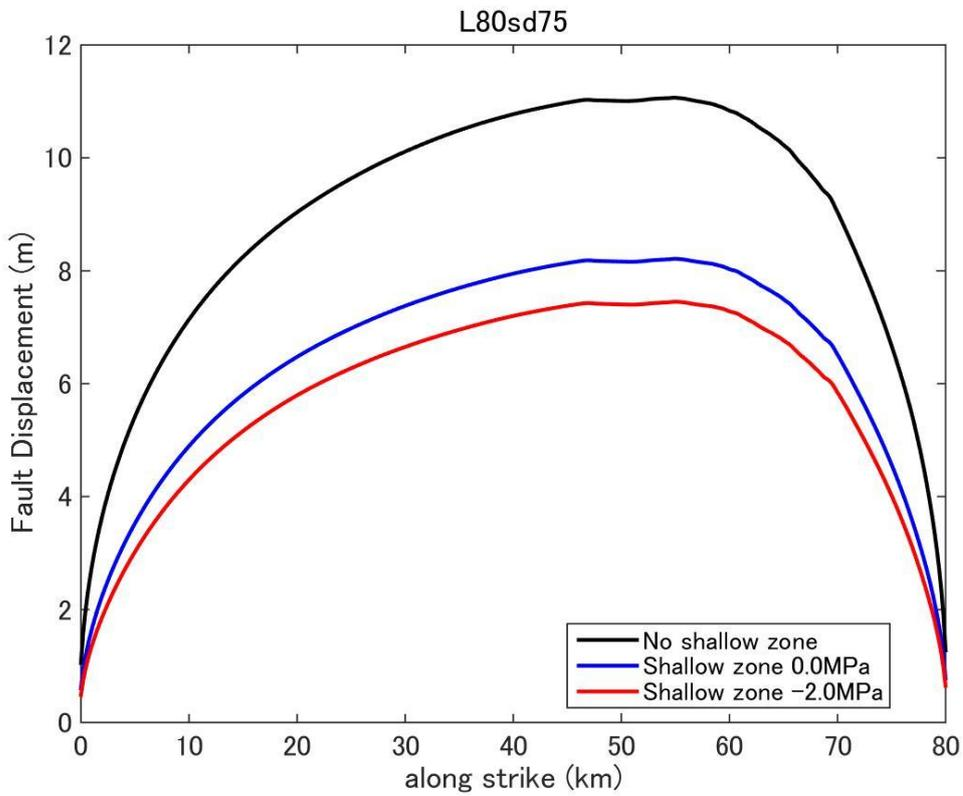
**Figure D24.** Fault displacement (surface rupture slip) distribution predicted by dynamic rupture model for a fault with fault length 80km and stress drop 7.5MPa.
