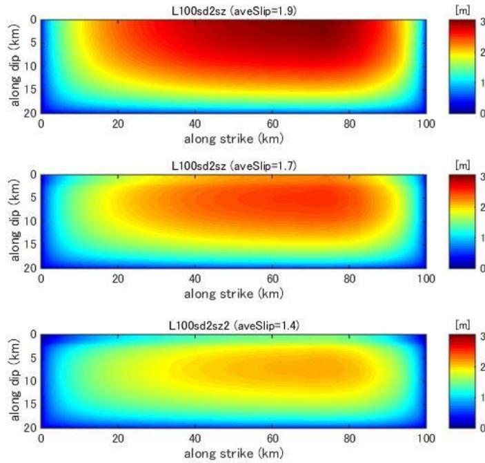
**Figure C25.** Final slip distribution predicted by dynamic rupture model for a fault with fault length 100km and stress drop 2.0MPa. [Top] no shallow zone model; [middle] weak shallow zone stress drop 0.0MPa; [bottom] weak shallow zone stress drop -2.0MPa.
