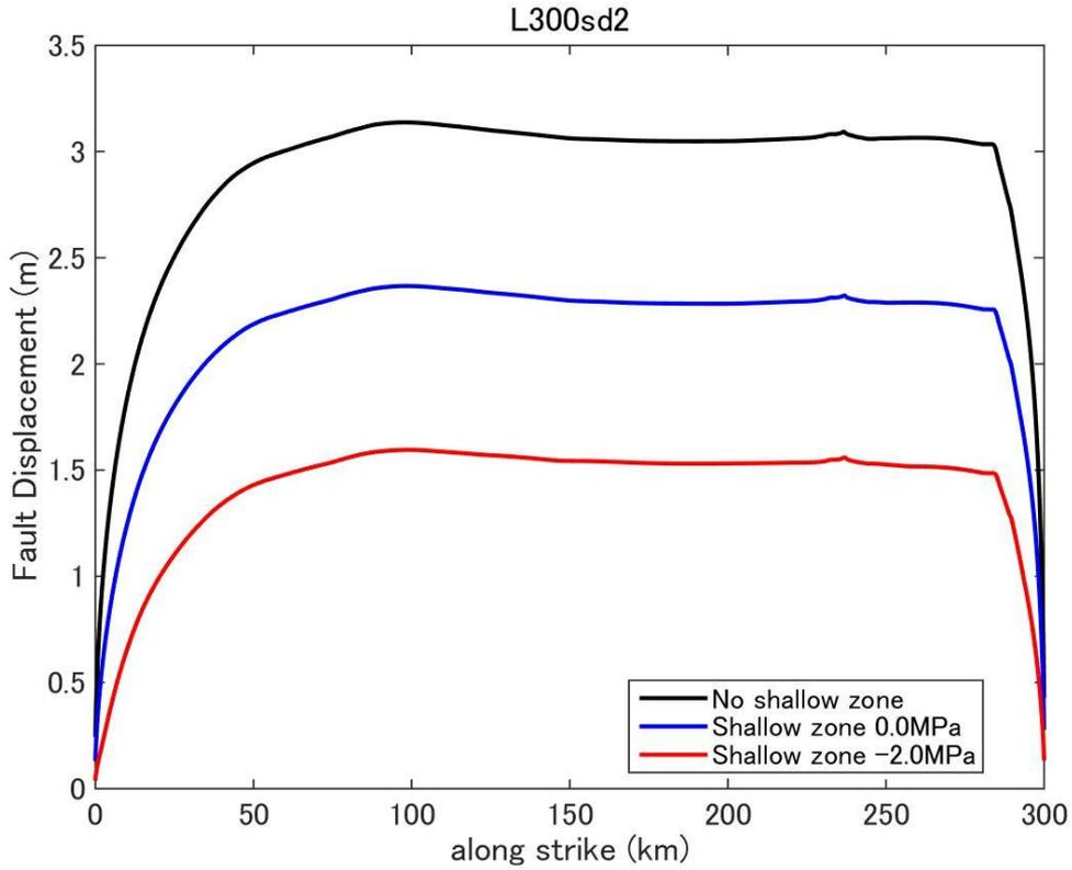
**Figure D43.** Fault displacement (surface rupture slip) distribution predicted by dynamic rupture model for a fault with fault length 300km and stress drop 2.0MPa.
