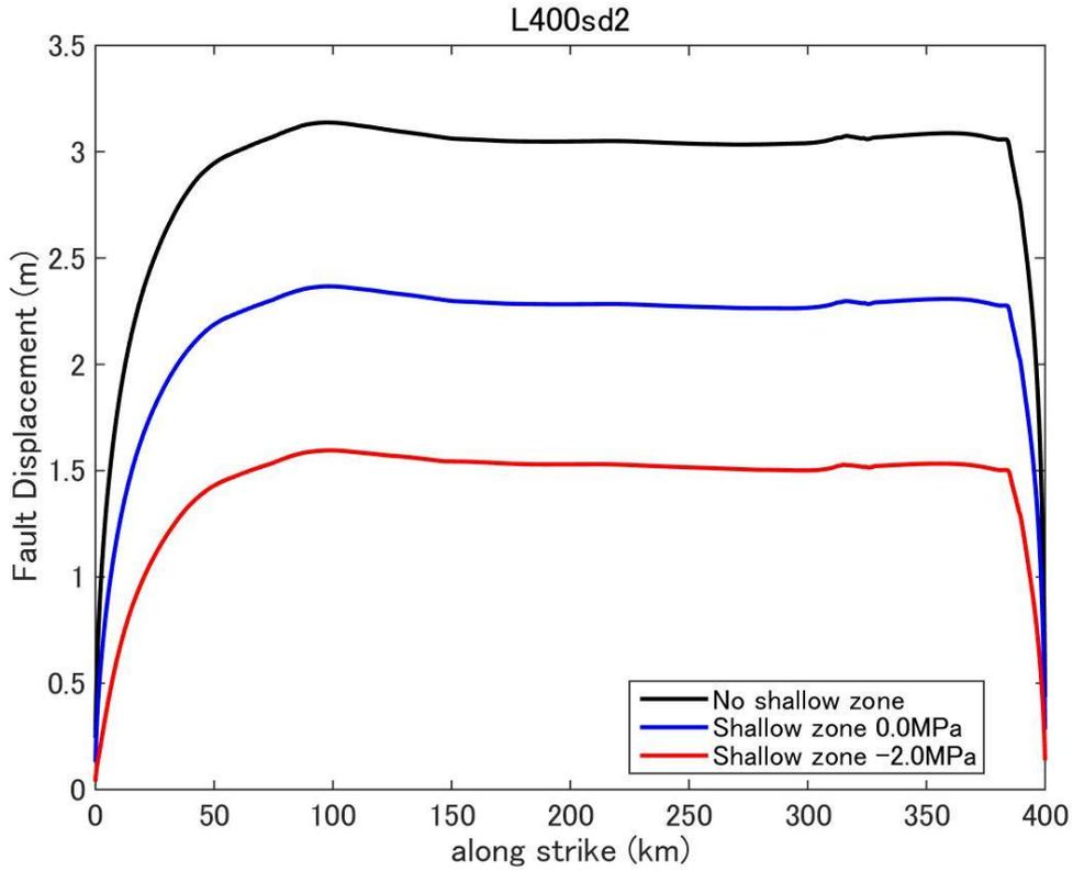
**Figure D49.** Fault displacement (surface rupture slip) distribution predicted by dynamic rupture model for a fault with fault length 400km and stress drop 2.0MPa.
