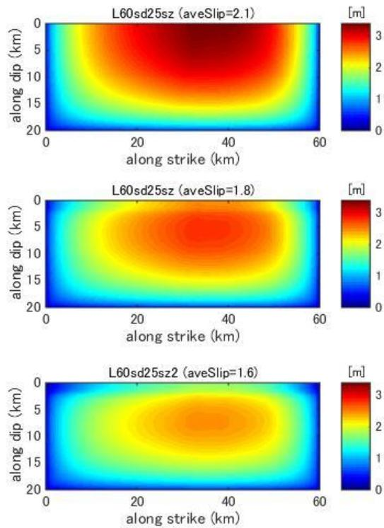
**Figure C16.** Final slip distribution predicted by dynamic rupture model for a fault with fault length 60km and stress drop 2.5MPa.
