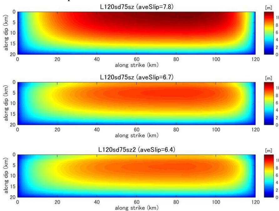
**Figure C36.** Final slip distribution predicted by dynamic rupture model for a fault with fault length 120km and stress drop 7.5MPa.
