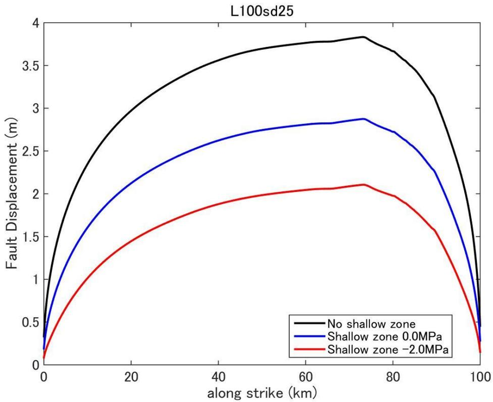
**Figure D28.** Fault displacement (surface rupture slip) distribution predicted by dynamic rupture model for a fault with fault length 100km and stress drop 2.5MPa.
