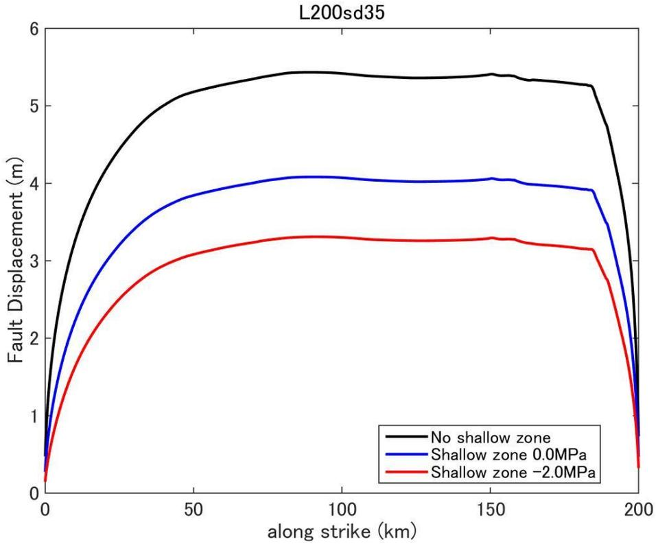
**Figure D41.** Fault displacement (surface rupture slip) distribution predicted by dynamic rupture model for a fault with fault length 200km and stress drop 3.5MPa.
