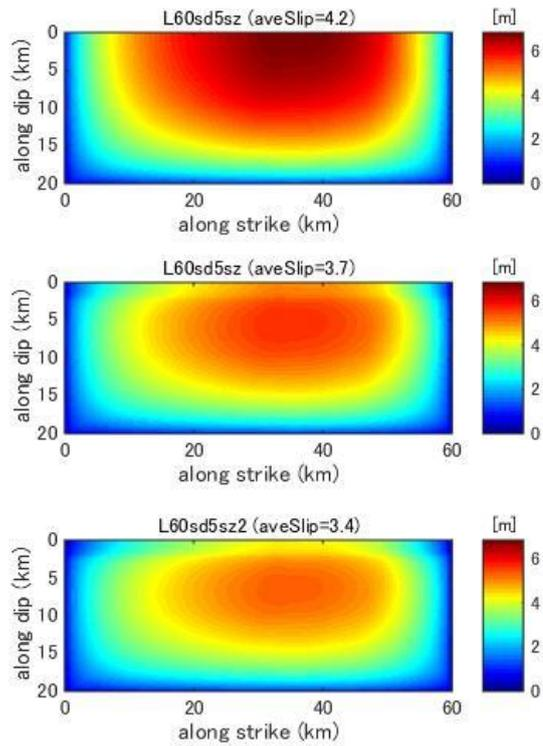
**Figure C15.** Final slip distribution predicted by dynamic rupture model for a fault with fault length 60km and stress drop 5.0MPa.
