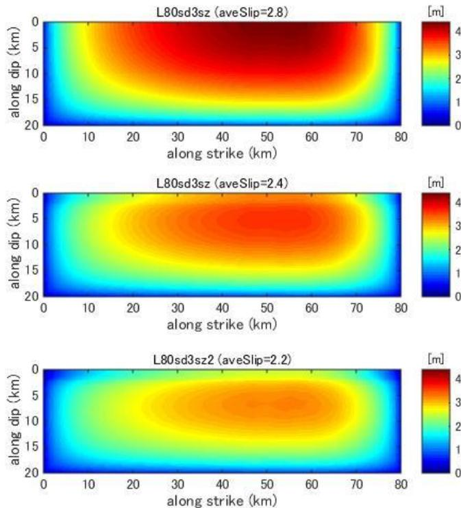
**Figure C20.** Final slip distribution predicted by dynamic rupture model for a fault with fault length 80km and stress drop 3.0MPa.
