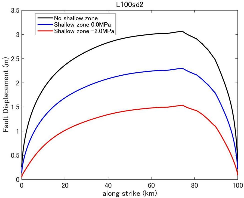
**Figure D25.** Fault displacement (surface rupture slip) distribution predicted by dynamic rupture model for a fault with fault length 100km and stress drop 2.0MPa.
