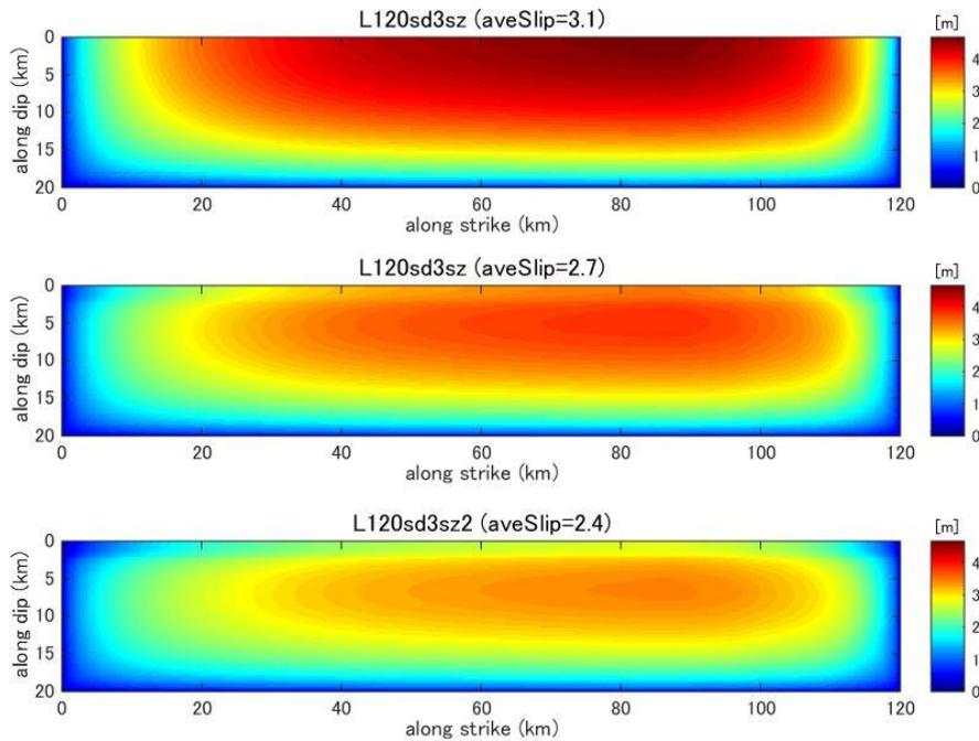
**Figure C32.** Final slip distribution predicted by dynamic rupture model for a fault with fault length 120km and stress drop 3.0MPa.
