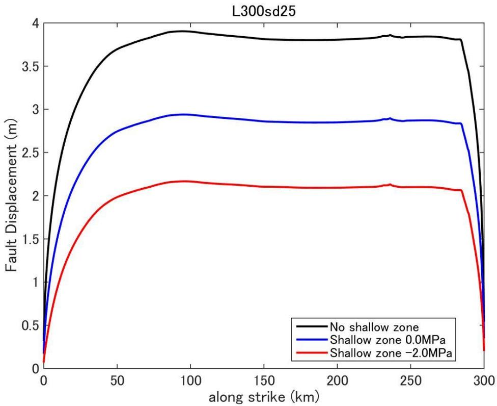
**Figure D46.** Fault displacement (surface rupture slip) distribution predicted by dynamic rupture model for a fault with fault length 300km and stress drop 2.5MPa.
