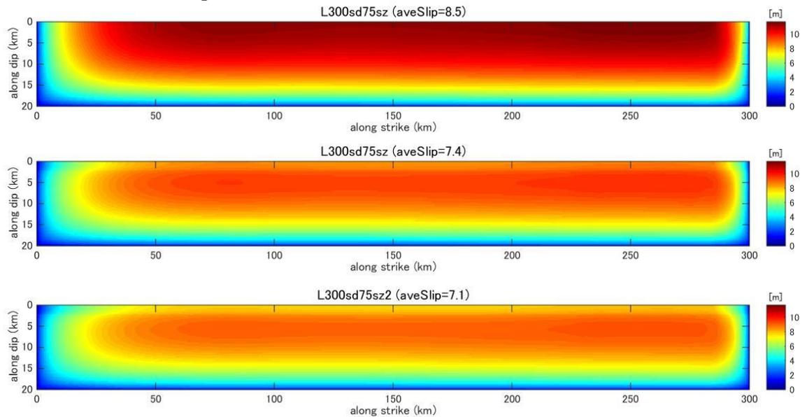
**Figure C48.** Final slip distribution predicted by dynamic rupture model for a fault with fault length 300km and stress drop 7.5MPa.
