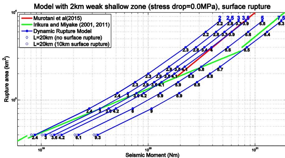
**Figure 13.** Models with weak shallow zone characterized with 0.0 MPa of stress drop:: Rupture area vs seismic moment for all the dynamic stress drop models and empirical models of Murotani et al (2015) and Irikura and Miyake (2001, 2011). The blue level at the end of each curve is the corresponding dynamic stress drop. The black number at each point is the static stress drop corresponding to each individual model.
