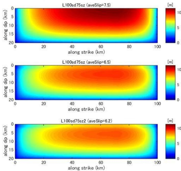
**Figure C30.** Final slip distribution predicted by dynamic rupture model for a fault with fault length 100km and stress drop 7.5MPa.
