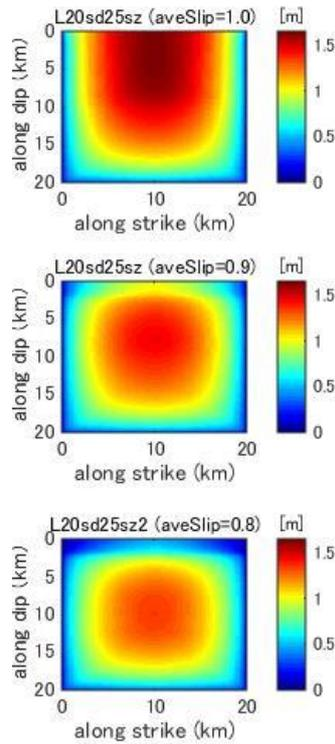
**Figure C4.** Final slip distribution predicted by dynamic rupture model for a fault with fault length 20km and stress drop 2.5MPa.
