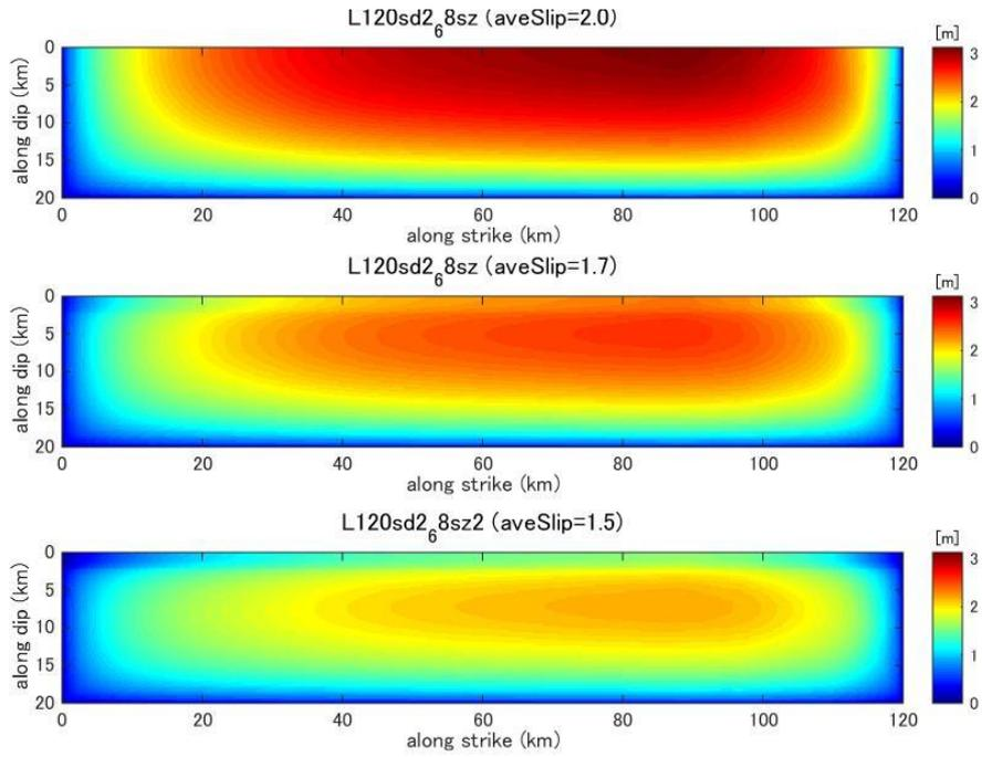
**Figure C31.** Final slip distribution predicted by dynamic rupture model for a fault with fault length 120km and stress drop 2.0MPa. [Top] no shallow zone model; [middle] weak shallow zone stress drop 0.0MPa; [bottom] weak shallow zone stress drop -2.0MPa.
