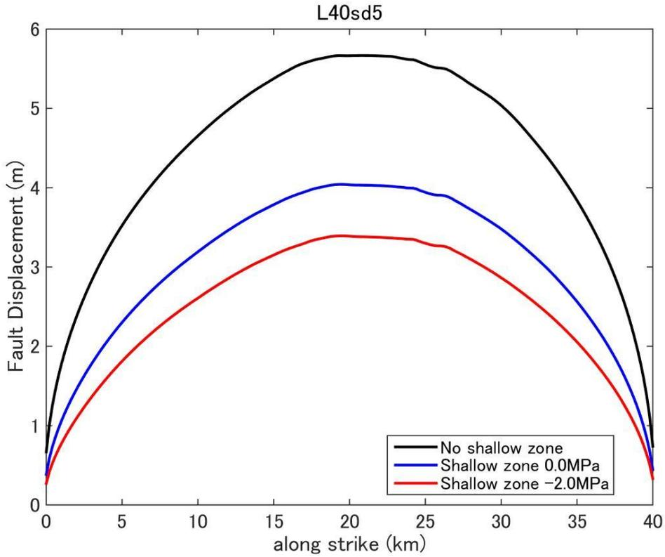
**Figure D9.** Fault displacement (surface rupture slip) distribution predicted by dynamic rupture model for a fault with fault length 40km and stress drop 5.0MPa.
