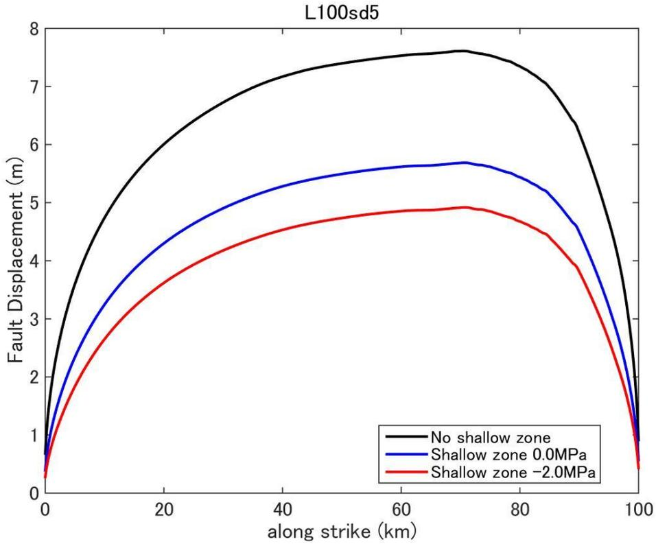
**Figure D27.** Fault displacement (surface rupture slip) distribution predicted by dynamic rupture model for a fault with fault length 100km and stress drop 5.0MPa.
