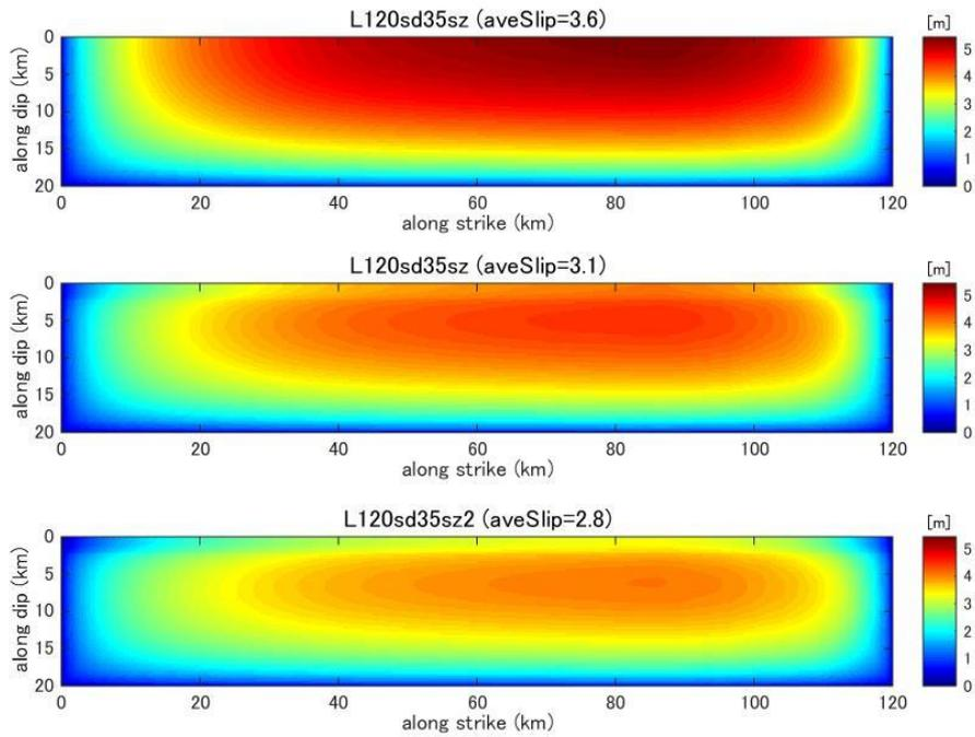
**Figure C35.** Final slip distribution predicted by dynamic rupture model for a fault with fault length 120km and stress drop 3.5MPa.
