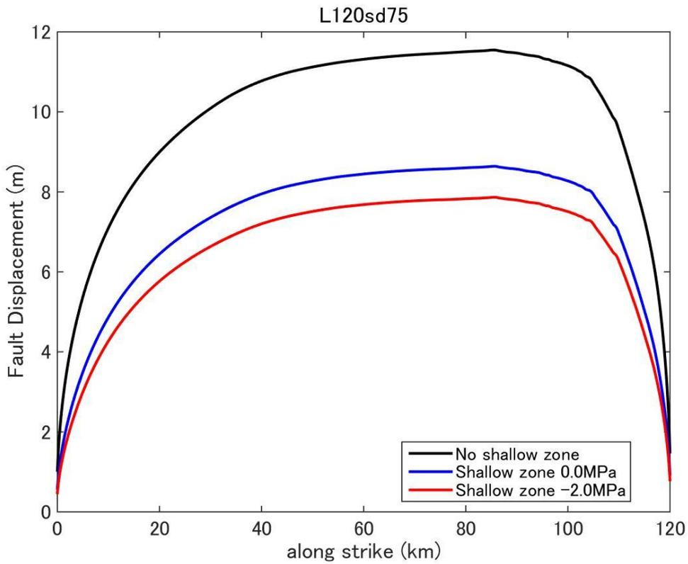
**Figure D36.** Fault displacement (surface rupture slip) distribution predicted by dynamic rupture model for a fault with fault length 120km and stress drop 7.5MPa.
