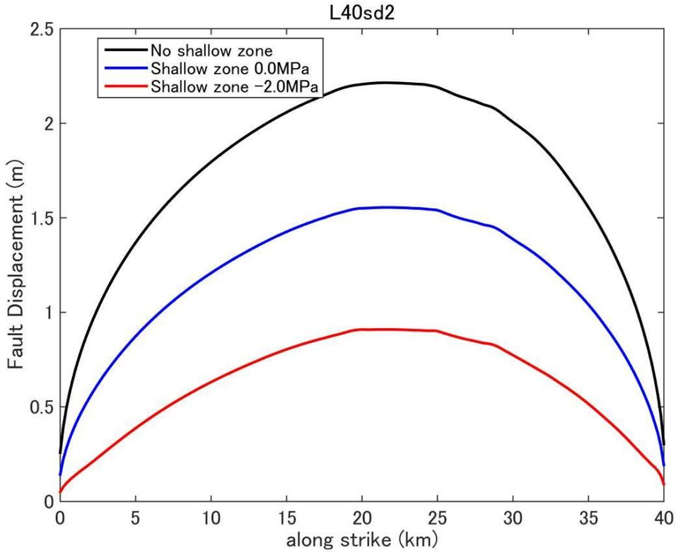
**Figure D7.** Fault displacement (surface rupture slip) distribution predicted by dynamic rupture model for a fault with fault length 40km and stress drop 2.0MPa.
