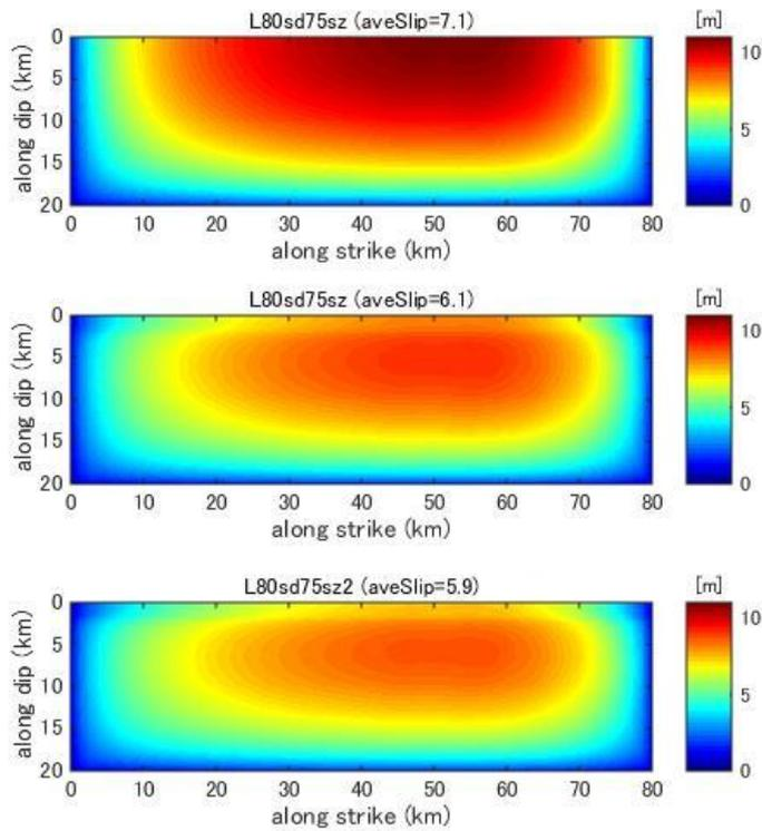
**Figure C24.** Final slip distribution predicted by dynamic rupture model for a fault with fault length 80km and stress drop 7.5MPa.
