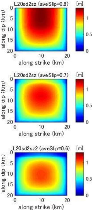
**Figure C1.** Final slip distribution predicted by dynamic rupture model for a fault with fault length 20km and stress drop 2.0MPa. [Top] no shallow zone model; [middle] weak shallow zone stress drop 0.0MPa; [bottom] weak shallow zone stress drop -2.0MPa.
