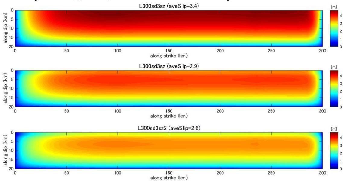
**Figure C44.** Final slip distribution predicted by dynamic rupture model for a fault with fault length 300km and stress drop 3.0MPa.
