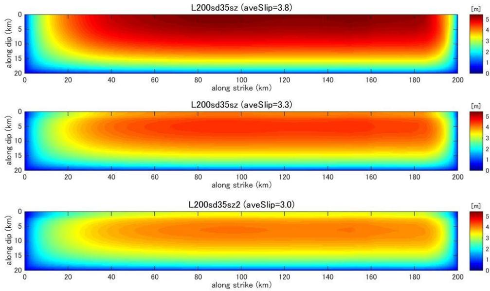
**Figure C41.** Final slip distribution predicted by dynamic rupture model for a fault with fault length 200km and stress drop 3.5MPa.
