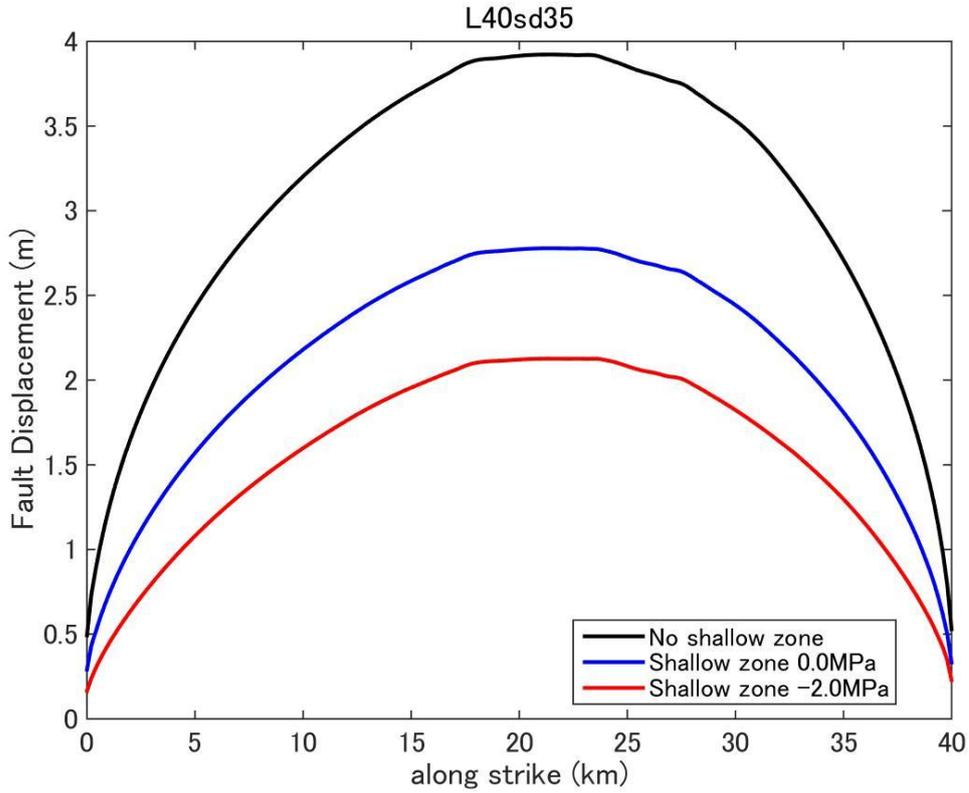
**Figure D11.** Fault displacement (surface rupture slip) distribution predicted by dynamic rupture model for a fault with fault length 40km and stress drop 3.5MPa.
