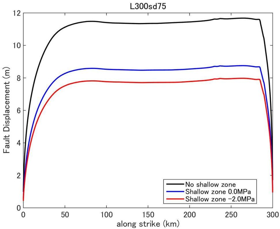
**Figure D48.** Fault displacement (surface rupture slip) distribution predicted by dynamic rupture model for a fault with fault length 300km and stress drop 7.5MPa.
