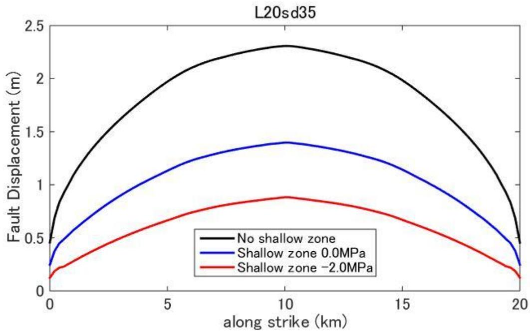
**Figure D5.** Fault displacement (surface rupture slip) distribution predicted by dynamic rupture model for a fault with fault length 20km and stress drop 3.5MPa.
