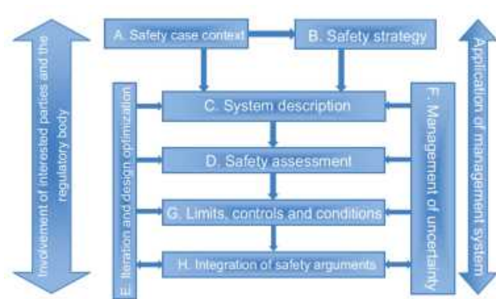
FIG. 3. Application of the management system and the process for interaction with the regulatory body and interested parties.
