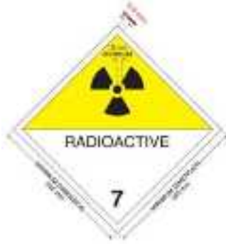
FIG.6. Placard. Except as permitted by para. 571, minimum dimensions shall be as shown and the minimum width of the line inside the edge forming the diamond shall be 5 mm ; when different dimensions are used, the relative proportions shall be maintained, The number '7' shall not be less than 25mm high. The background colour of the upper half of the label shall be yellow and the lower half white, the colour of the trefoil and the printing shall be black. The use of word "RADIOACTIVE" in the bottom half is optional, to allow the alternative use of this placard to display the appropriate UN number for the consignment.
