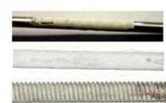
Fig. 11 Typical fouling pictures of smooth and finned tubes for a heat flux of 200 kW/m 2 and a given concentration of 1.6 g/L
