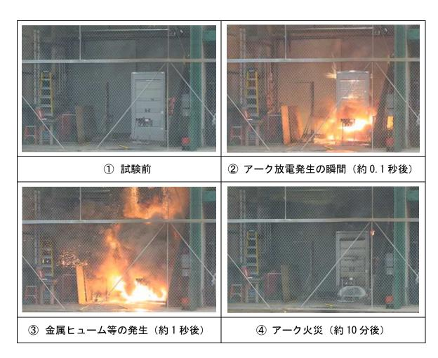
図4.2 配電盤のHEAF 試験 Fig. 4.2 HEAF test of distribution panel
