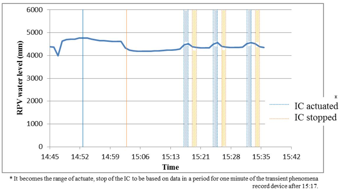
Figure 1.2 Behavior of RPV Water Level (including IC actuation and stop timing)
