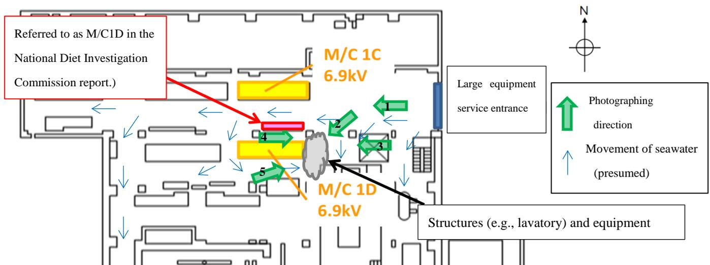
Figure 2.21 Layout Plan of the Turbine Building's 1st Floor of Unit 1<sup>30</sup>
