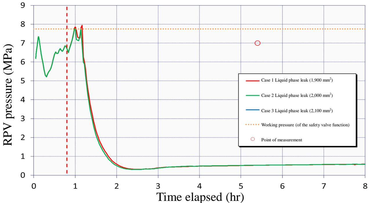
Figure 4.4 Behavior of RPV Pressure (cases with leak from the liquid phase)
