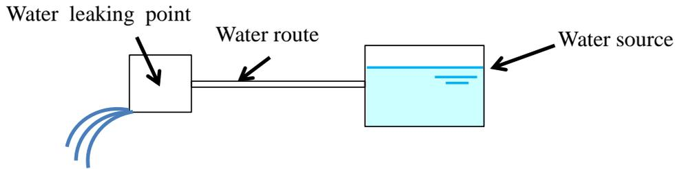
Figure 3.1 Relation between Water Leaking Point, Water Route, and Water Source (image diagram)
