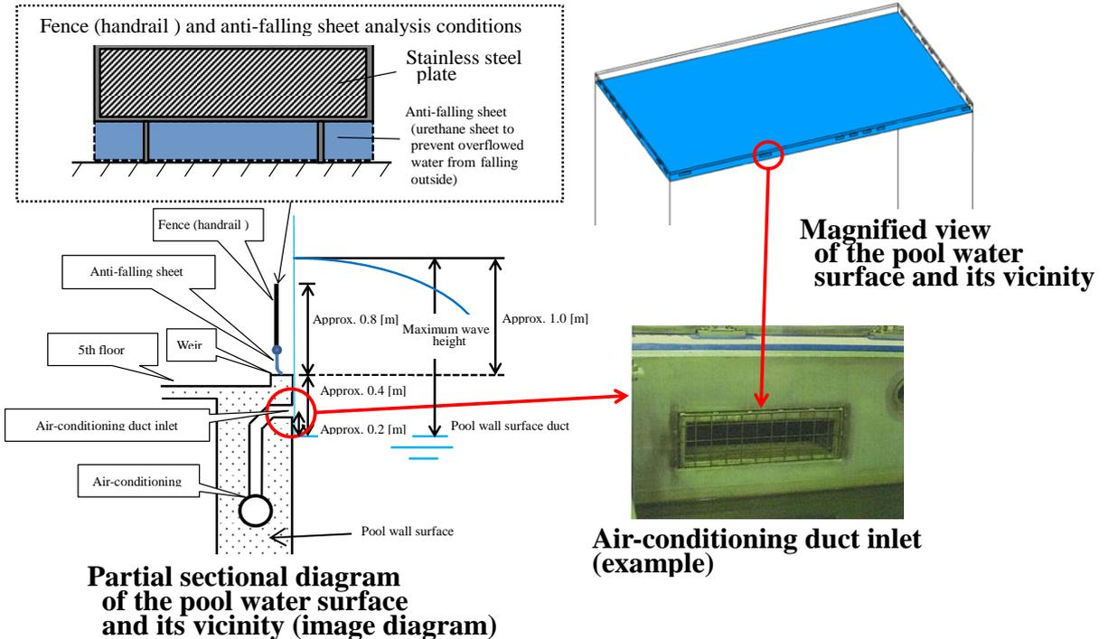
Figure 3.11 Slushing Analysis Conditions (2)
