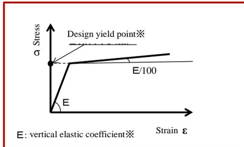
**Stress-strain diagram considering panels, etc.**
