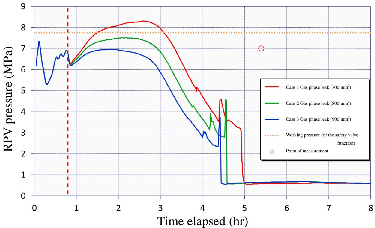
Figure 4.3 Behavior of RPV Pressure (cases with leak from the gas phase)
