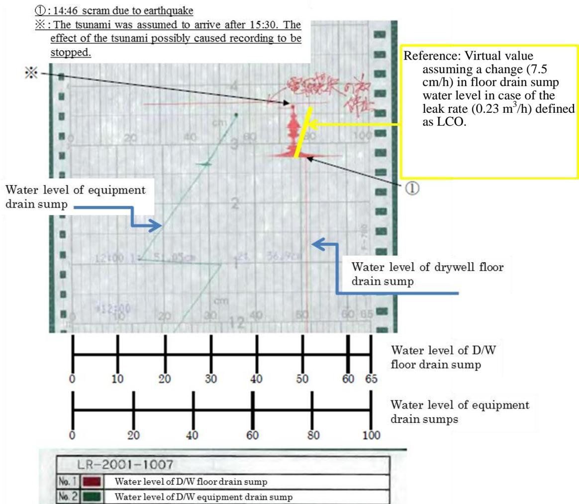
Figure 1.3 Water Levels of Drywell Floor Drain Sumps and Equipment Drain Sumps <sup>5</sup>
