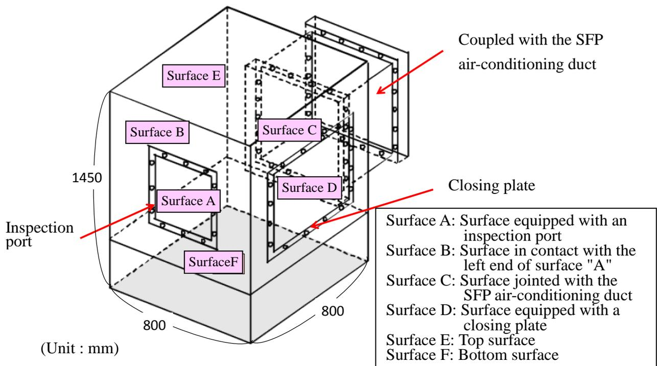
Figure 3.7 Structure of the Overflow Chamber (image diagram)
