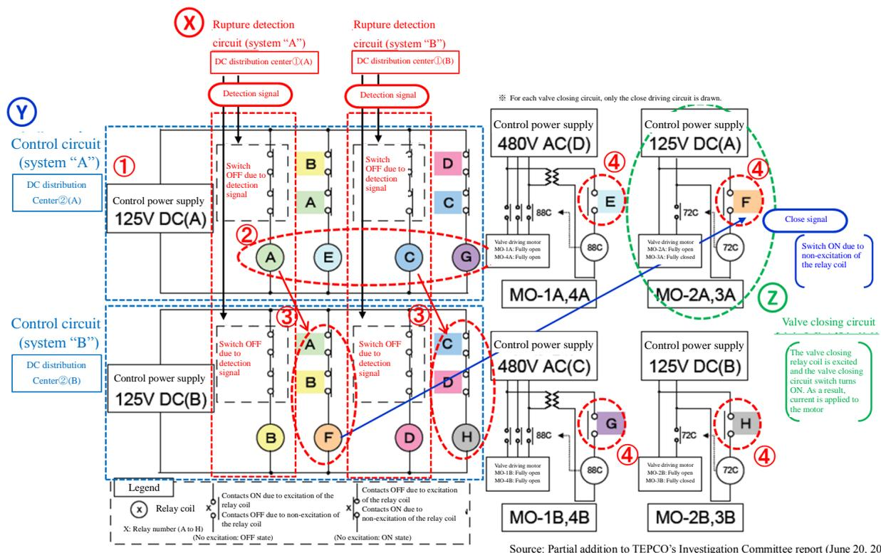
Figure 5.8 IC Isolation Valve Working Mechanism in case of Controlling Power Loss (operation logic "B")
