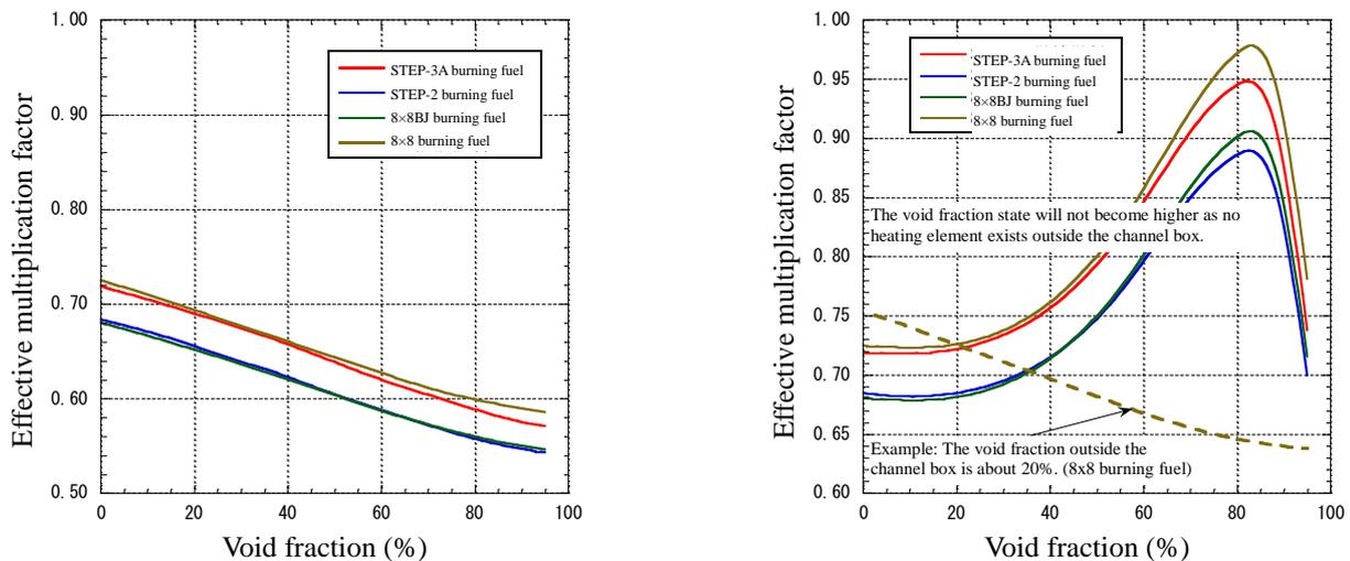
(a) Change of the void fraction only inside the channel box      (b) Change of the void fraction inside and outside the channel box (very conservative assumption)
