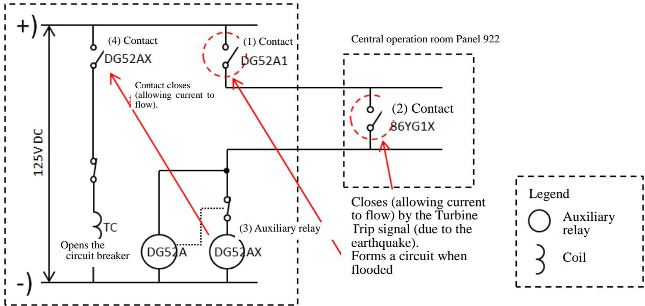
Figure 2.18 D/G1A Control Circuit Diagram
