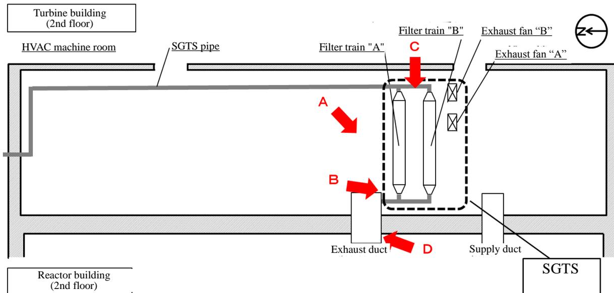
Figure 7.7 Layout of the SGTS Filter Trains, etc.
