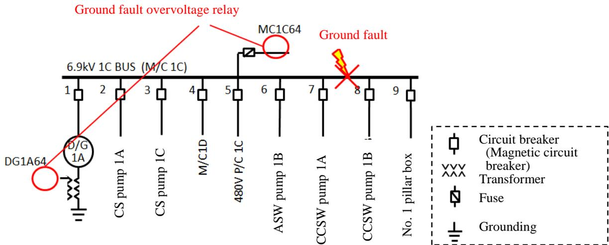
Figure 2.16 Electrical Connections for MC1C64 and DG1A64
