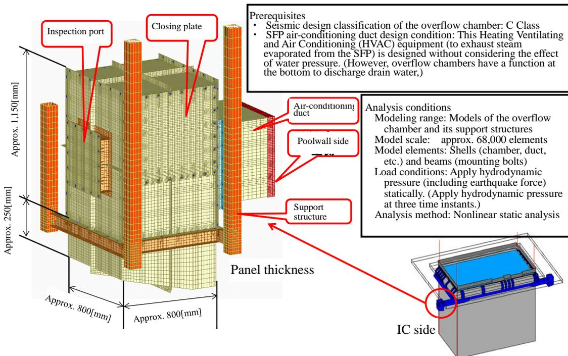
Figure 3.15 Overflow Chamber Deformation Evaluation Conditions (1)
