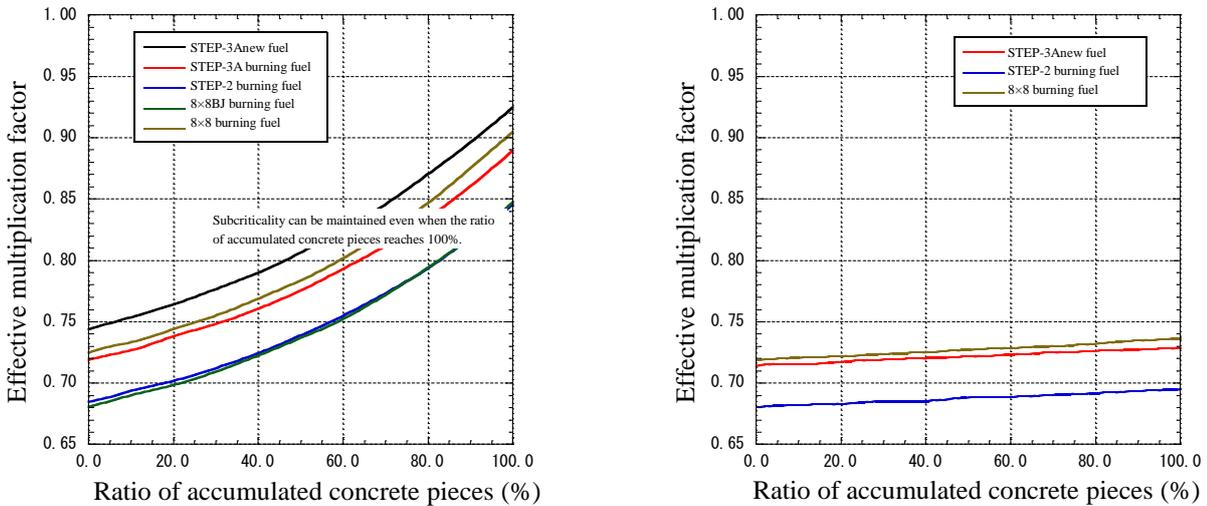
(a) When fuel assemblies are installed in an aluminum rack (b) When fuel assemblies are installed in a boron-added aluminum rack
