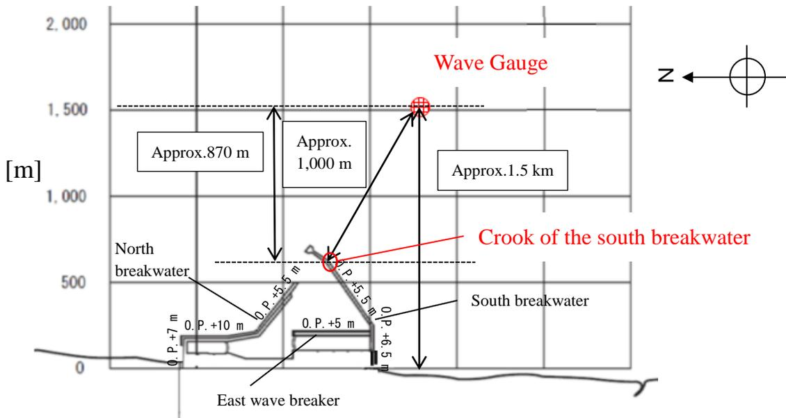
Figure 2.23 Location of the Wave Gauge, Distance between the Meter and the Premises, Breakwater Heights, etc.
