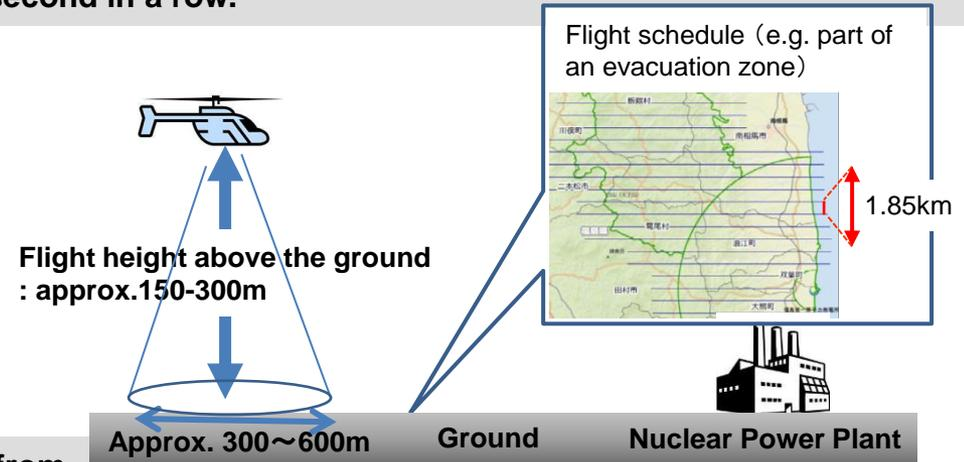
Setting up the given points on the ground, gamma rays from these points were measured from the upper sky at different heights.
