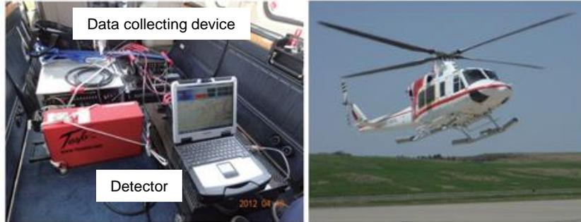
Airborne monitoring devices (left) are installed in a helicopter (right)
